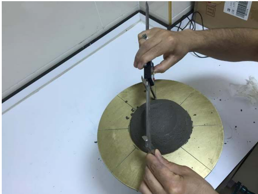
Figure 2 Photographic view flow test
