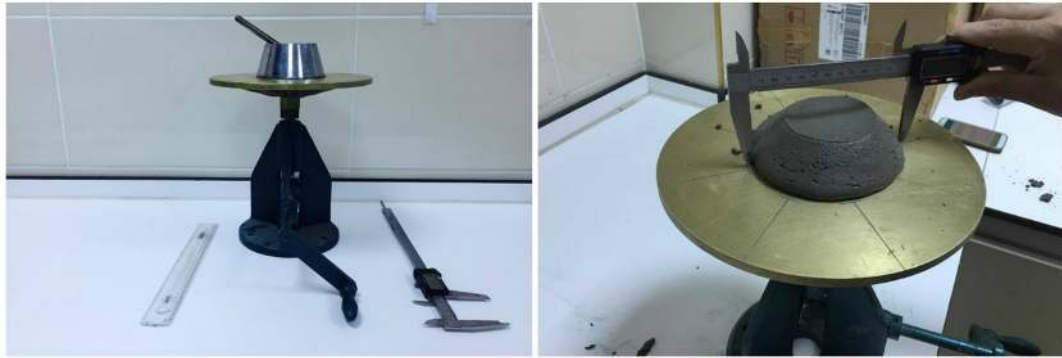
Figure 3.7 Flow table test
