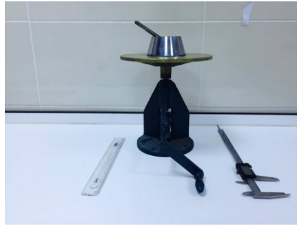
Figure 3.10 Flow table test
