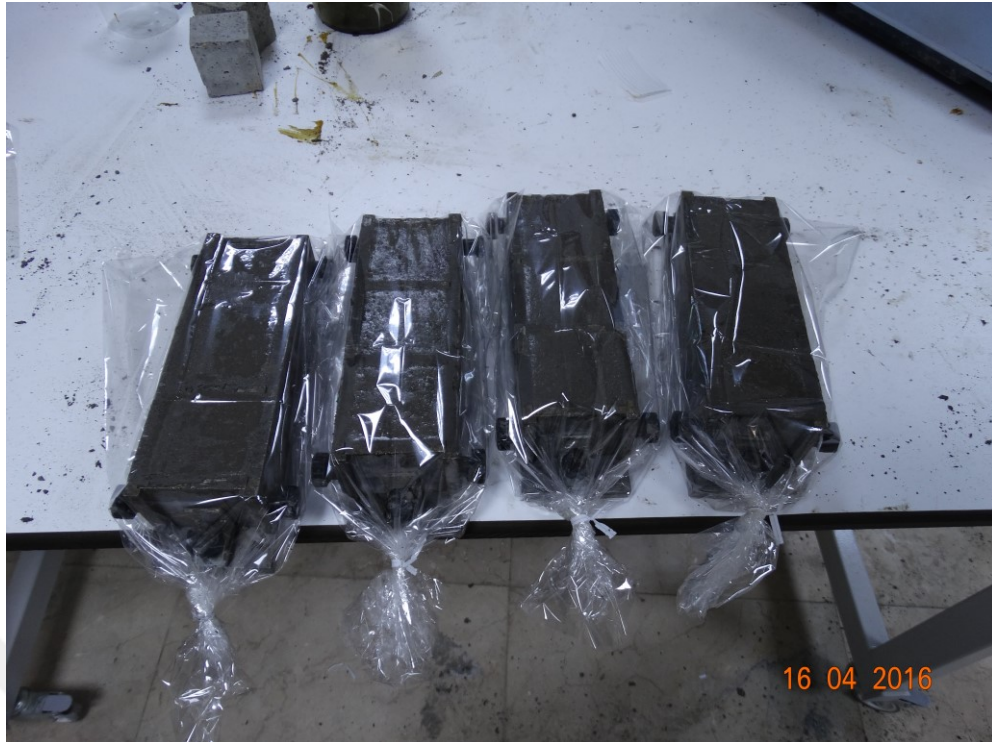
Figure 5 Photographic view of sealing the molds.
