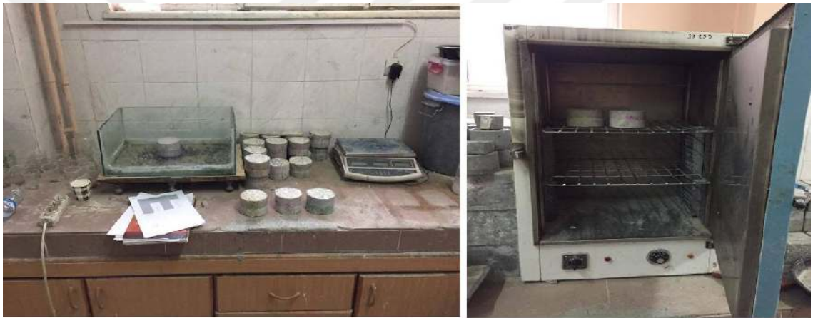
Figure 3.2 Photos of water sorptivity measurement
