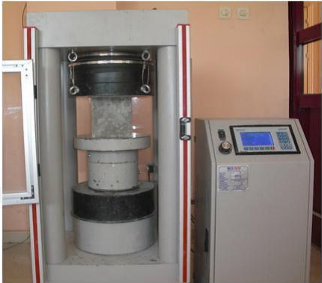
Figure 3.8 Compressive strength test
