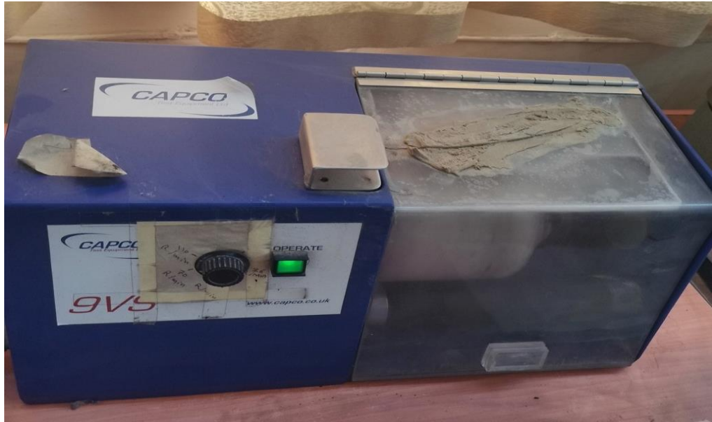
Figure 3.3 A laboratory mill containing metallic balls
