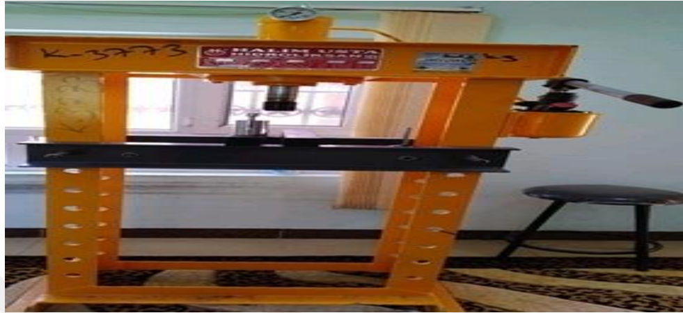
Figure 3.9 Hydraulic compaction of HALIM USTA
