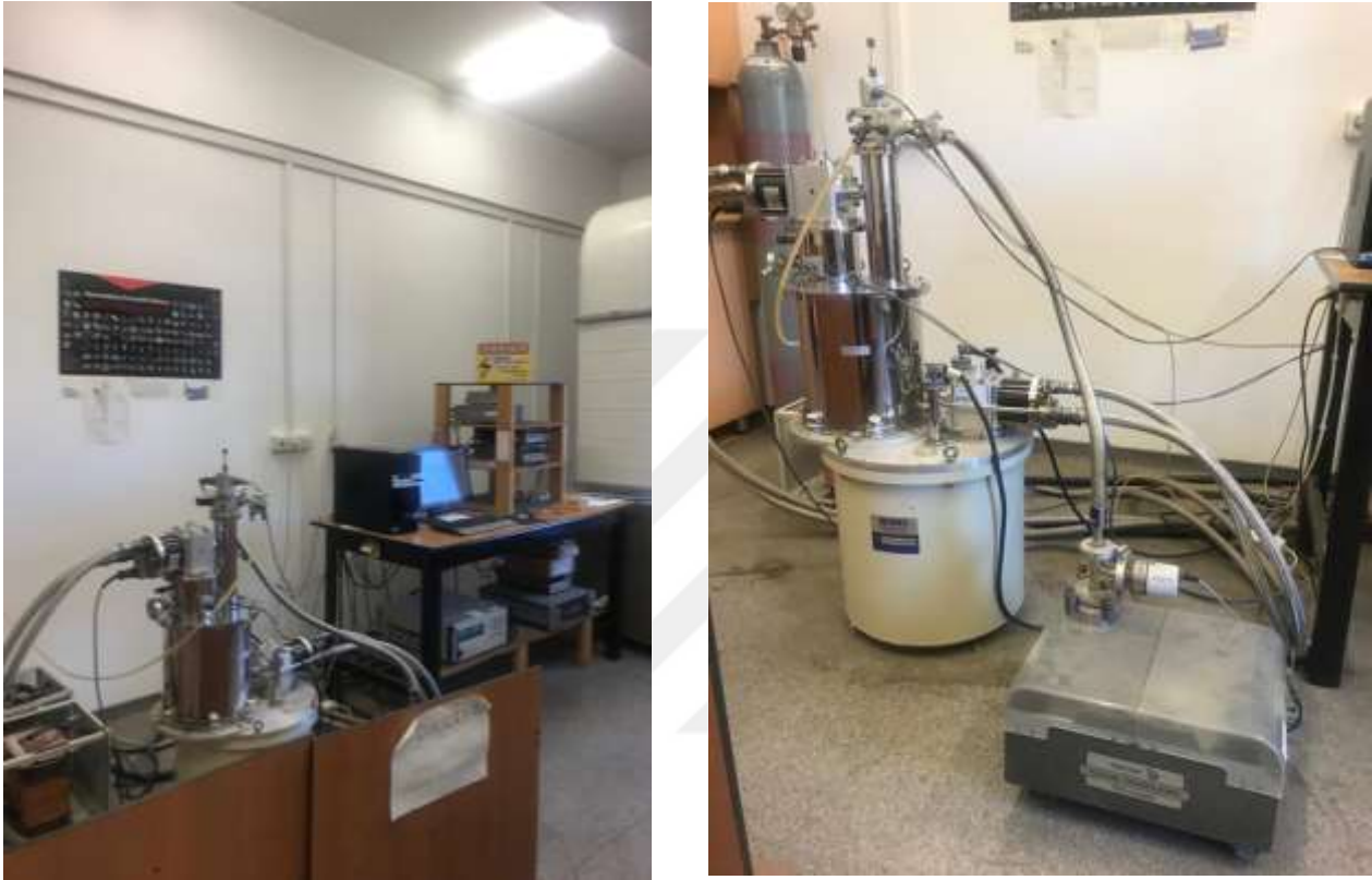
Picture 2.3. He-gas contact cryocooler and integrated into a superconducting coil magnet
