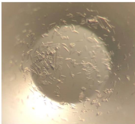
Figure 3.2.2: The microscope picture of hexahistidine tagged Nmar_0274 protein crystals. The crystals were obtained by microbatch under paraffin oil crystallization method at ambient temperature. Table 3.2.2 indicates the sparse matrix crystallization condition used to obtain Nmar_0274 protein crystals.
