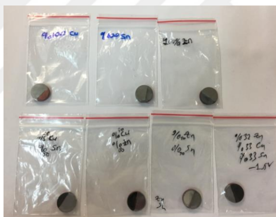
Figure 3.5 Photographs of steels electrodeposited by Cu, Sn, Zn, Cu-Sn, Cu-Zn, Zn-Sn, Cu-Zn-Sn; respectively
