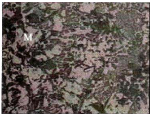
Magnetite and bicalcium silicate
