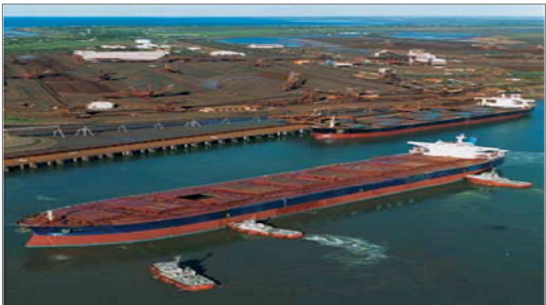
Figure 3.5 A typical picture of ship loading. Ships can carry about 170,000 tons of iron ore (Skillings Mining Review, 1996).
