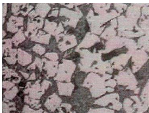
Magnetite filled by bicalcium silicate and calcium ferrite
