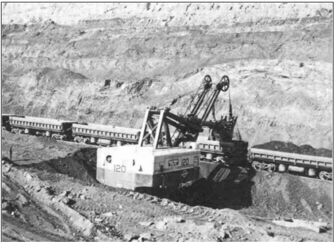
Figure 3.3 Electric power shovel on caterpillar tracks, making a sinking cut and loading ore into steel dump cars for haulage from an open pit mine to a beneficiation plant. Diesel-electric locomotives handle the dump cars while a cable carries power to the shovel (Hartmur et al., 1999).
