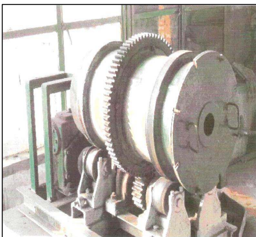
Drum mixer ( \Phi 280mm X 600mm, 32r/min)
