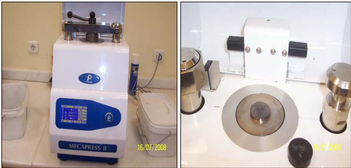
Figure 7.32 Hardening of sintered samples with epoxy resin.
