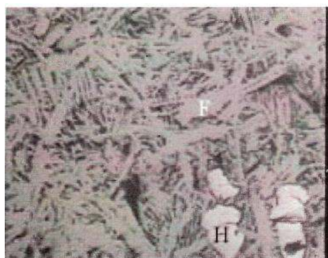
Bulk particles of hematite consolidated by interwoven texture
