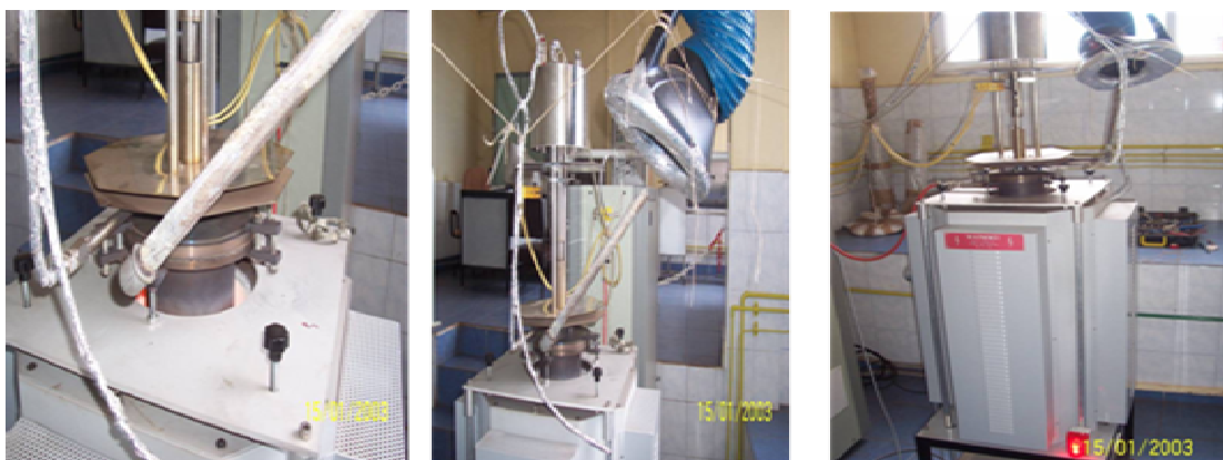
Figure 6.3 A picture of reduction under load testing device.
