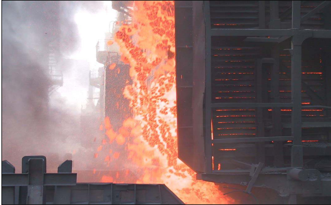
Figure 2.1 A general view of the coke oven. The oven has just been “pushed” and railroad car is full of incandescent coke that will now be taken to the “quench station” (Isdemir, 2010).
