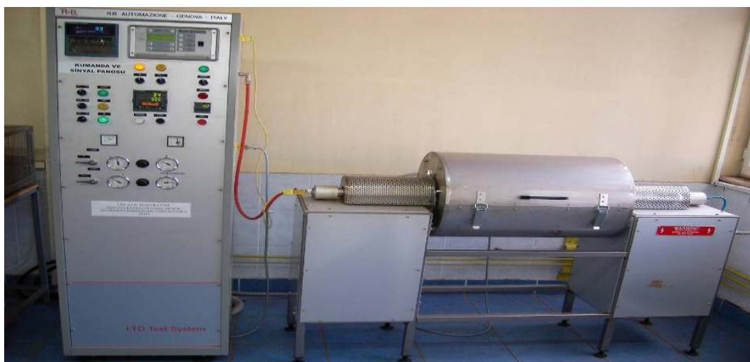
Figure 6.6 A picture of low temperature reduction disintegration testing device.
