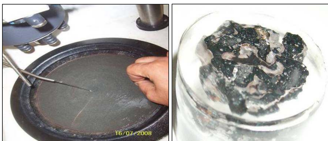
Figure 7.31 Sintered samples prepared for mineralogical analysis.
