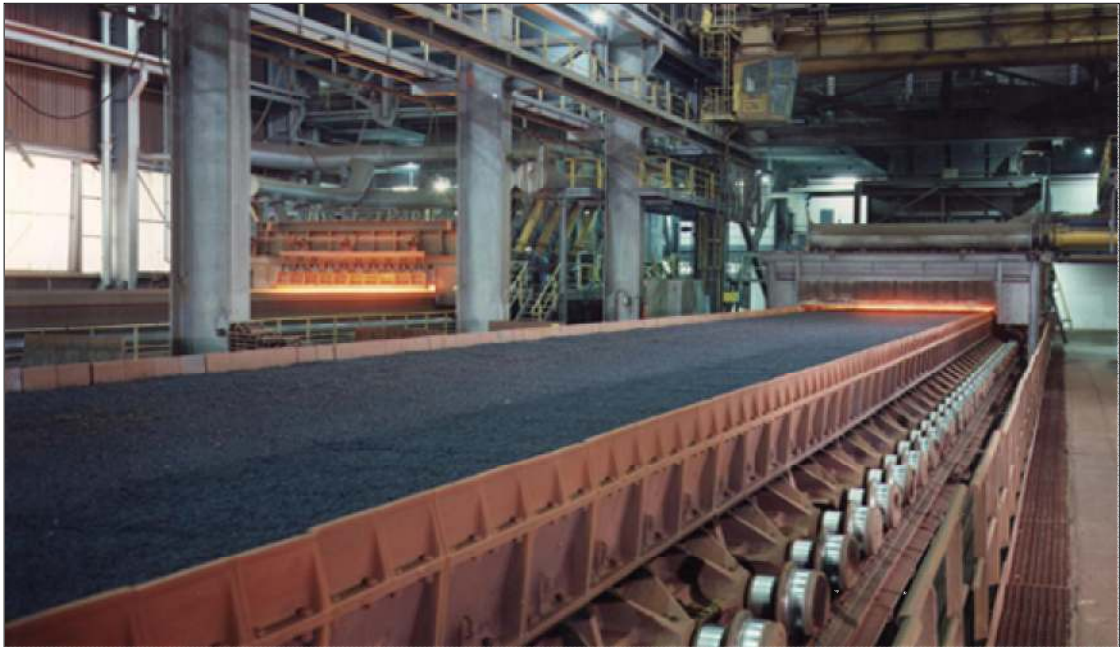
Figure 5.2 Photograph of a sinter strand with the charging facility (drums or chutes) and the ignition canopy at the starting end (Integrated Pollution Prevention and Control [IPPC], 2001).
