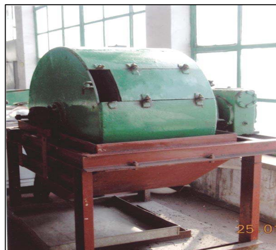
ISO Tumbler drum ( \Phi 1000 mm X 100 mm 25 r/min)
