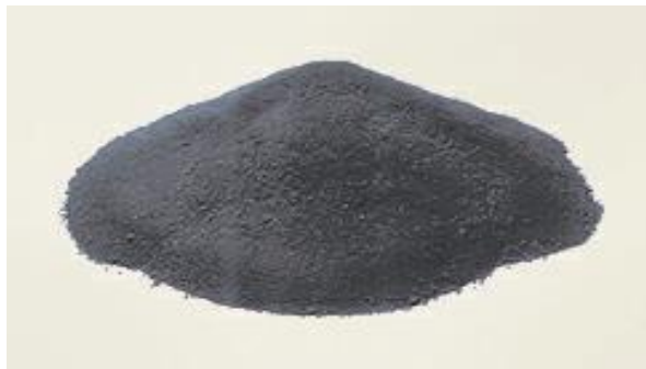
Figure 4.2 Photographic view of silica fume.
