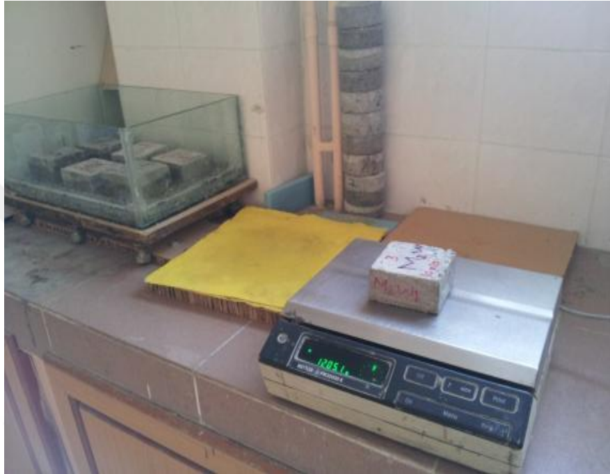
Figure B 1 Photographic view of weight reading by sensitive balance
