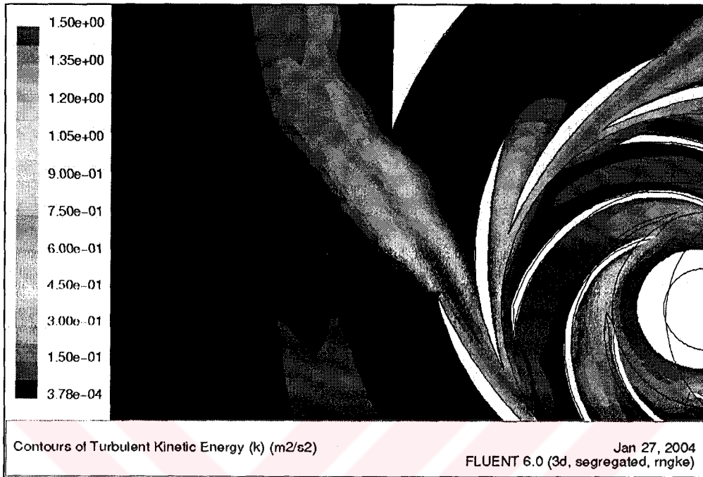
Figure 4.25 a) Contours of static pressure b) Contours of velocity magnitude c) Velocity vectors d) Contours of vorticity magnitude e) Contours of TKE (for 3.48 1/s) – Case III
