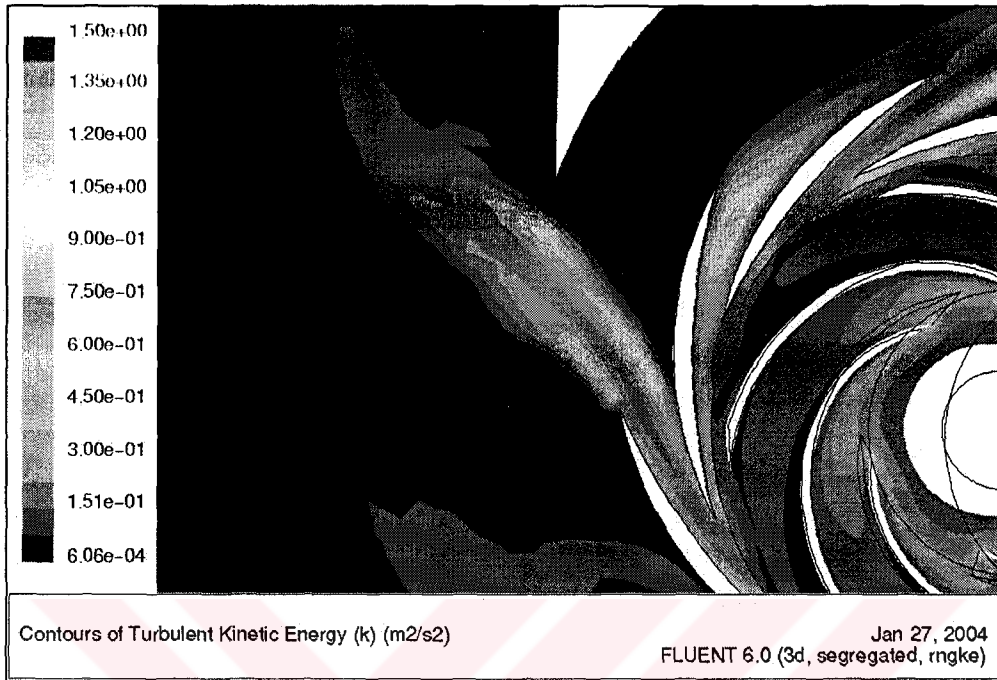
Figure 4.24 a) Contours of static pressure b) Contours of velocity magnitude c) Velocity vectors d) Contours of vorticity magnitude e) Contours of TKE (for 4.12 l/s) – Case III
