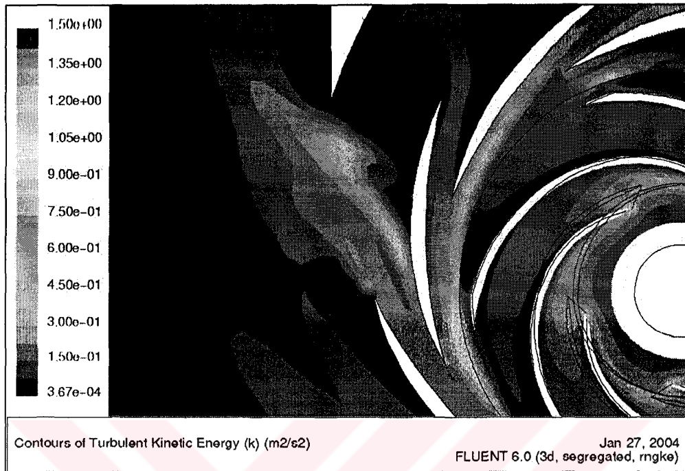
Figure 4.19 a) Contours of static pressure b) Contours of velocity magnitude c) Velocity vectors d) Contours of vorticity magnitude e) Contours of TKE (for 4.12 l/s) – Case I
