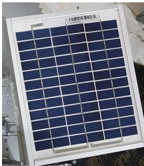
Figure 3.1 Polycrystalline Silicon PV panel
