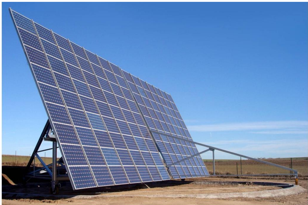
Figure 2.12 Azimuth-Altitude Dual Axis Tracker, Toledo, Spain [41]
