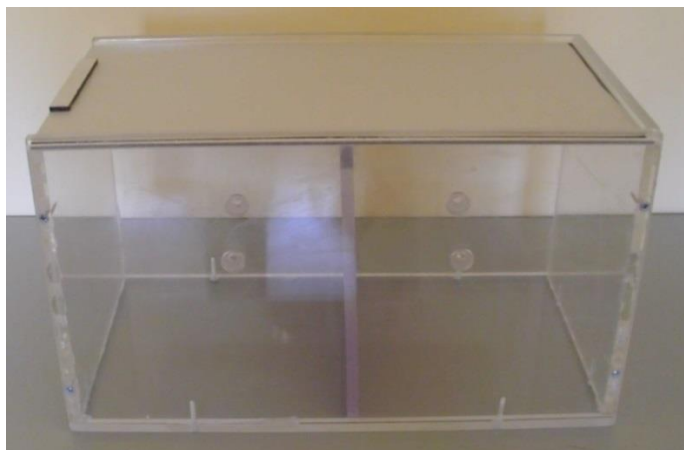
Figure 3. 11 Plexiglass testing apparatus
