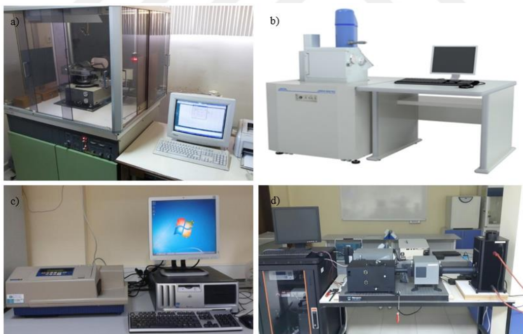
Figure 3.14. Photographs of the characterization devices of (a) Rigaku D/Max-IIIC diffractometer (b) JEOL JSM-6610 SEM ( https://www.jeol.co.jp/en/products/detail/JSM-6610series.html ) (c) SpectraMax M5 and (d) Dongwoo Optron.
