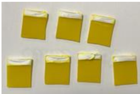
Figure 3.7. CdS nanospheres grown by two steps on ITO coated glass substrates.
