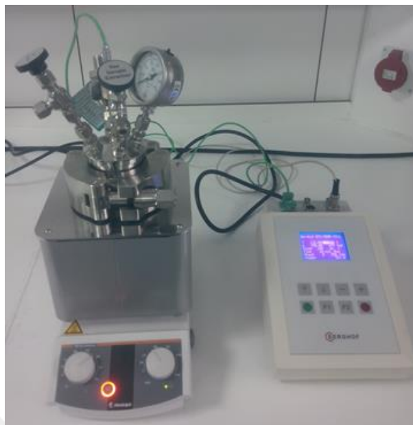
Figure 3.6. Hydrothermal system used to produce CdS nanospheres.
