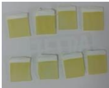
Figure 3.4. CdS thin films grown by chemical bath deposition on ITO coated glass substrates.
