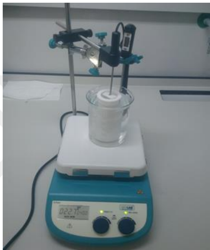
Figure 3.3. Chemical bath deposition system used to produce CdS thin film.
