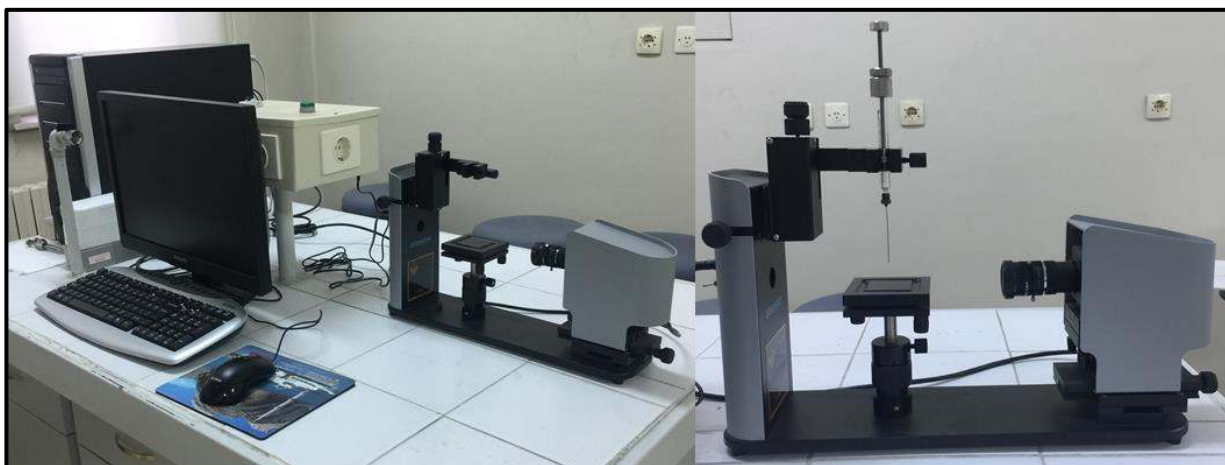
Figure 3.12 Surface tension measurement device (Attension Theta®)
