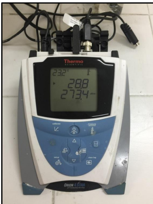
Figure 3.11 Conductivity measurement device (Orion 4 Star Plus®)
