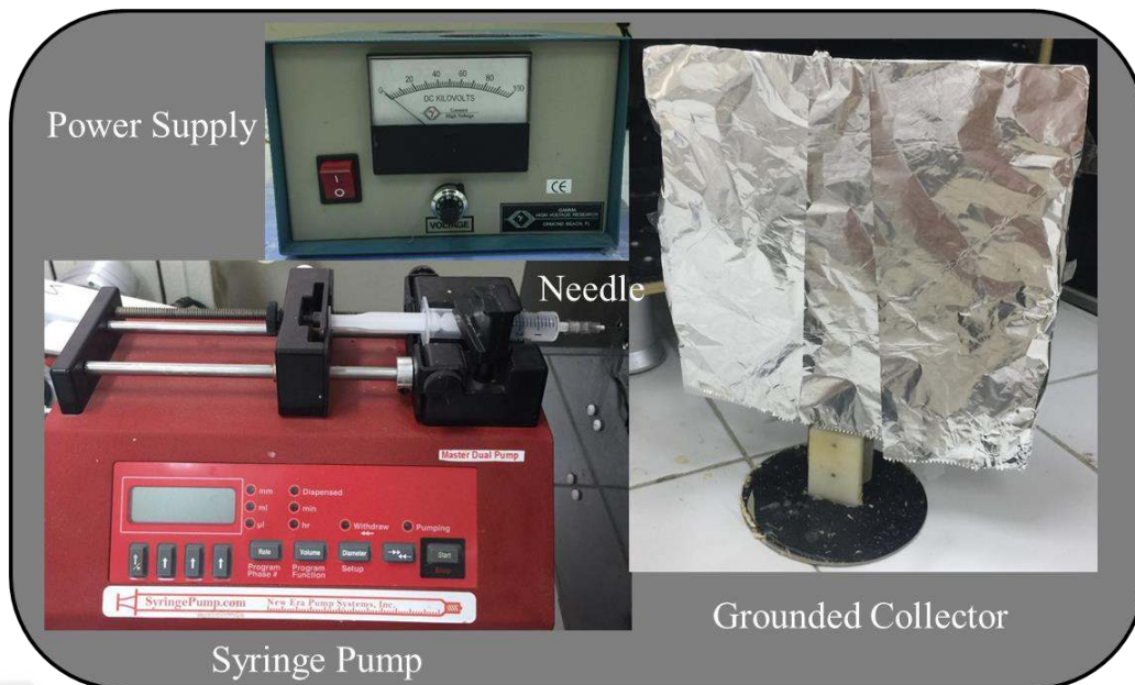
Figure 1.5 Basic components of electrospraying method
