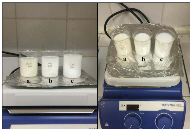
Figure 3.5 Macrosilicone Softener Solution and Preparation; a) Pure concentration Macrosilicone Softener solution, b) 1:5 concentration Macrosilicone Softener solution c) 1:10 concentration Macrosilicone Softener solution
