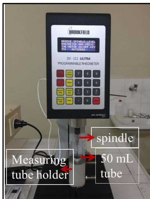
Figure 3.10 Viscosity measurement device (Brookfield DV-3 Ultra®)
