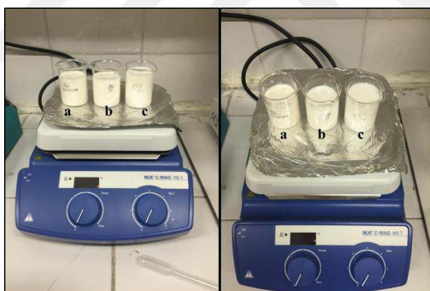
Figure 3.8 Fluorocarbon&Dendrimer Solution and Preparation; a) Pure concentration Fluorocarbon&Dendrimer solution, b) 1:5 concentration Fluorocarbon&Dendrimer solution c) 1:10 concentration Fluorocarbon&Dendrimer solution
