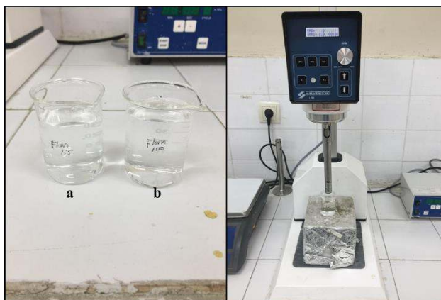
Figure 3.9 Flame Retardant Solution and Preparation; a) 1:5 concentration Fluorocarbon&Dendrimer solution b) 1:10 concentration Fluorocarbon&Dendrimer solution
