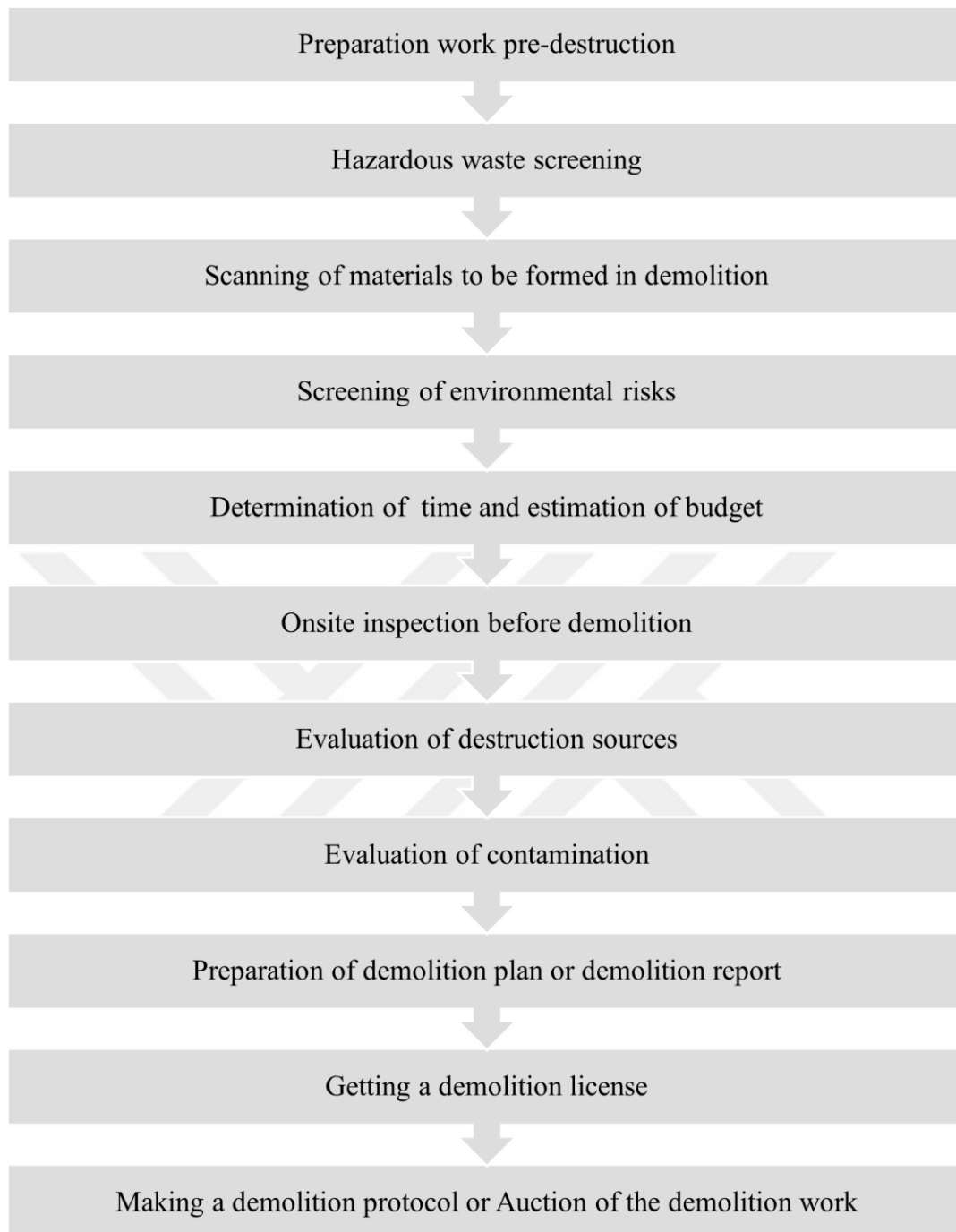
Figure 3.2 Steps of demolition process
