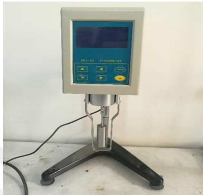
Figure 3.20: NDJ-5S Viscometer Measuring Device for Dynamic Viscosity of Nanofluid.
