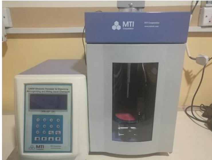
Figure 3.19: 1200W Ultrasonic Processor for Homogenizing Nanofluid Produced by MTI CORPORATION.
