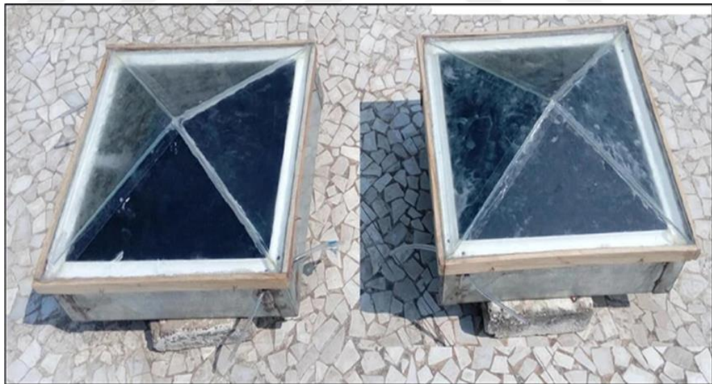
Figure 2.7: The Experimental Models Of The Square Hierarchical Solar Distiller [35].
