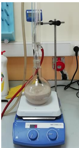
Figure 2.2. Large scale silylation process using reflux apparatus
