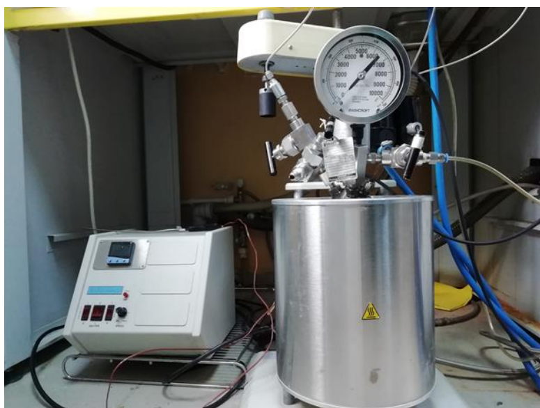
Figure 2.5. The heater and the high pressure reactor
