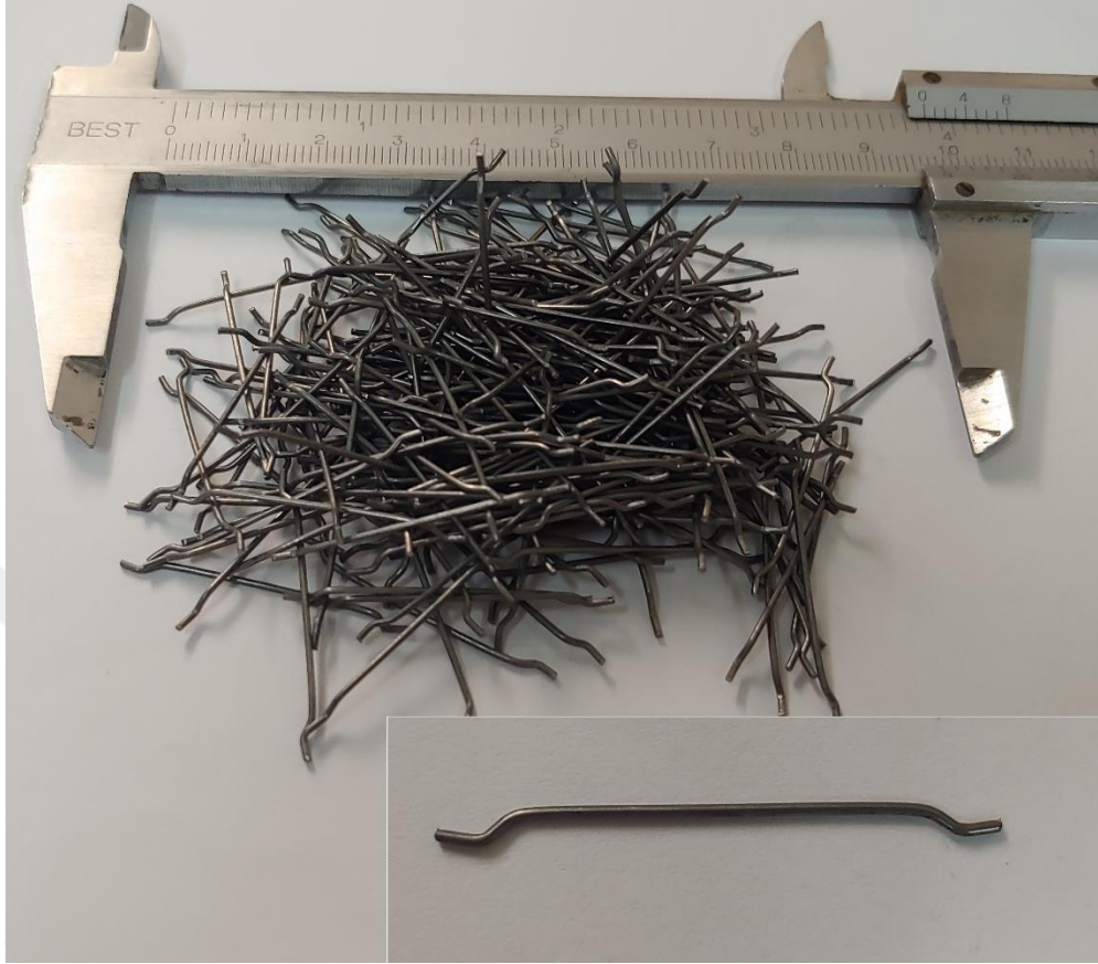
Figure 3.3 Steel fibers (Personal archive, 2022)
