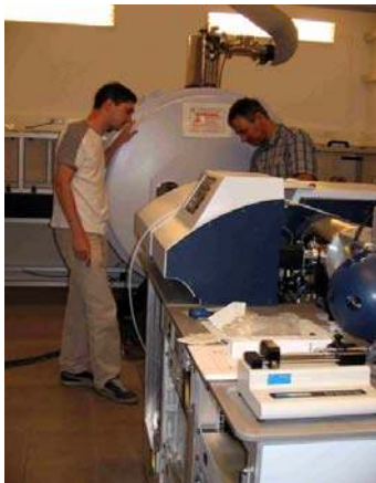
Resim 7.2. FT-ICR kütle spektrometresi (Fourier Transform Ion Cyclotron Resonance)
