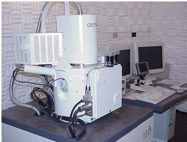
Resim 5.3. SEM cihazı (Silcox Research Group, Cornell University)
