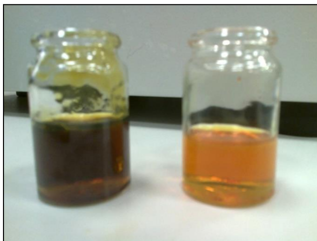
Figure 3-16 HVGO feed and the reaction product of a sample test with a commercial catalyst.
