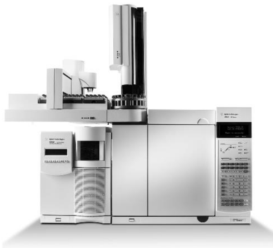
Figure 3-9 Agilent 6890N - 5975C GC-MS Instrument (retrieved from http://www.chem-agilent.com/cimg/5975C_7693A-224x90.jpg )
