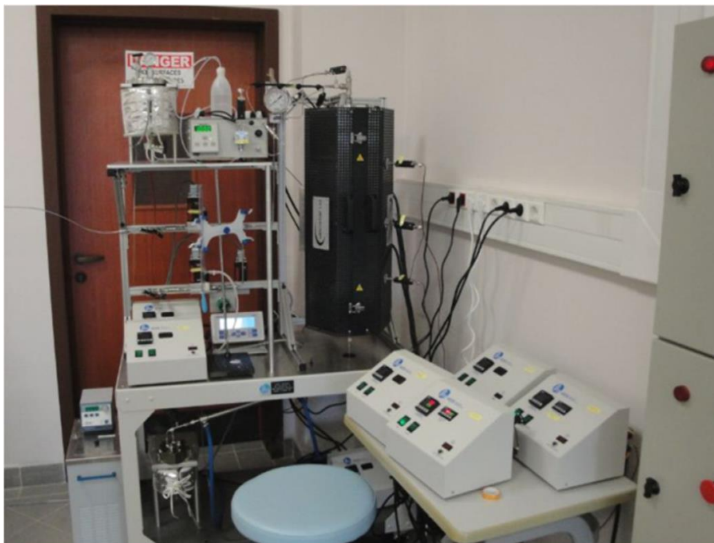
Figure 3-2 Parr custom made reactor system used in catalysts testing.
