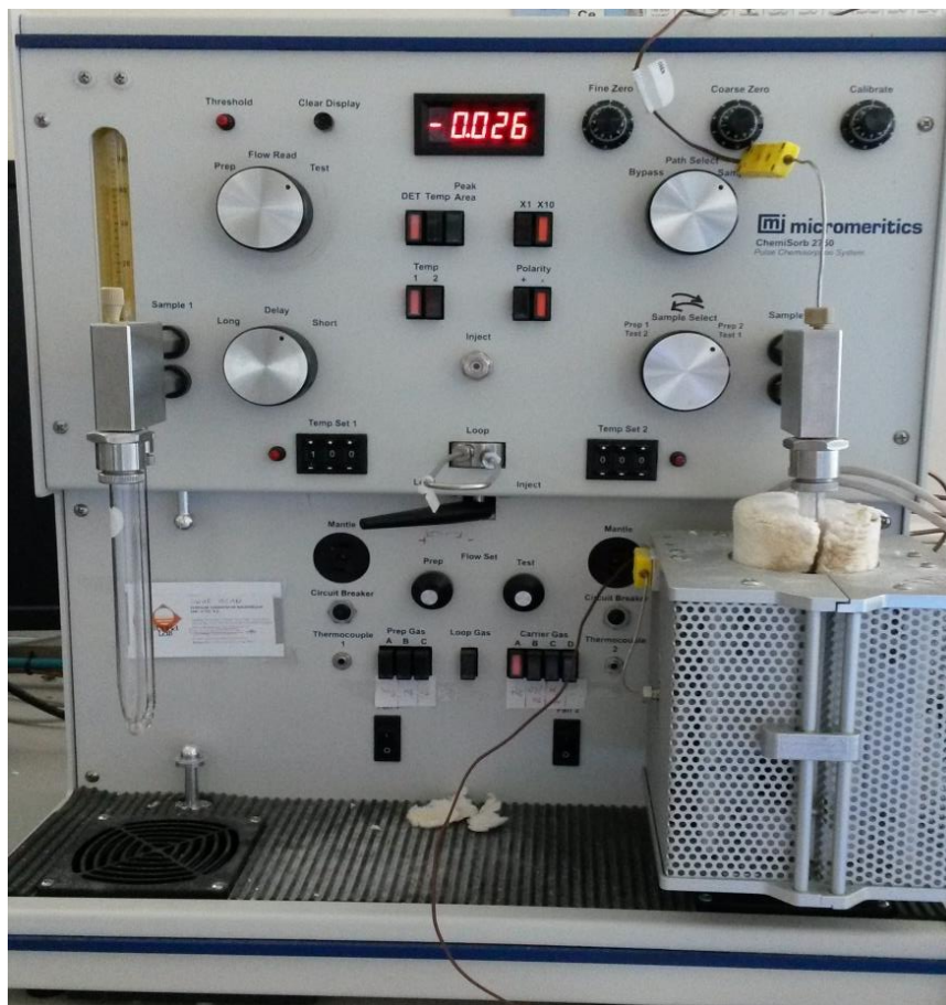
Figure 3-7 Chemisorb 2750 (Micromeritics) apparatus.
