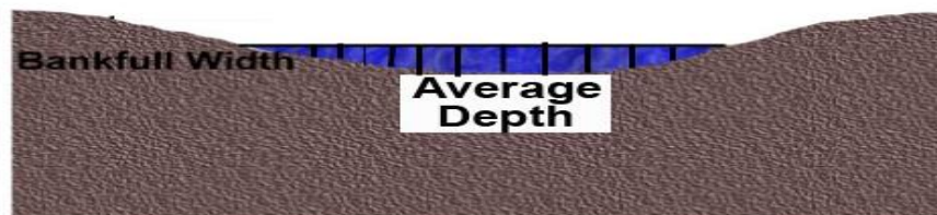
Figure 2.10 : Representative demonstration and calculation of width/depth ratio.
