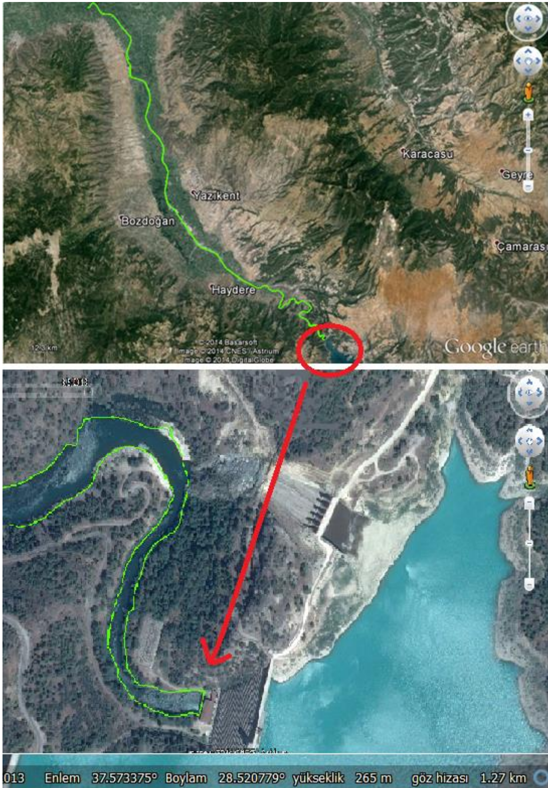
Figure 3.9 : Example selection step of the unregulated reach in BMW via zooming-in and excluding a dam. (Google Earth, 2014)
