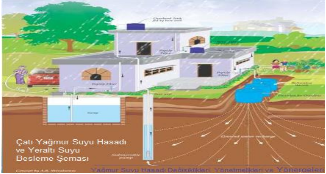
Şekil 3.2.5.a Yağmur suyu hasat sistemi (bangalore water supply and sewerage board, karnataka gazette, 2010)
