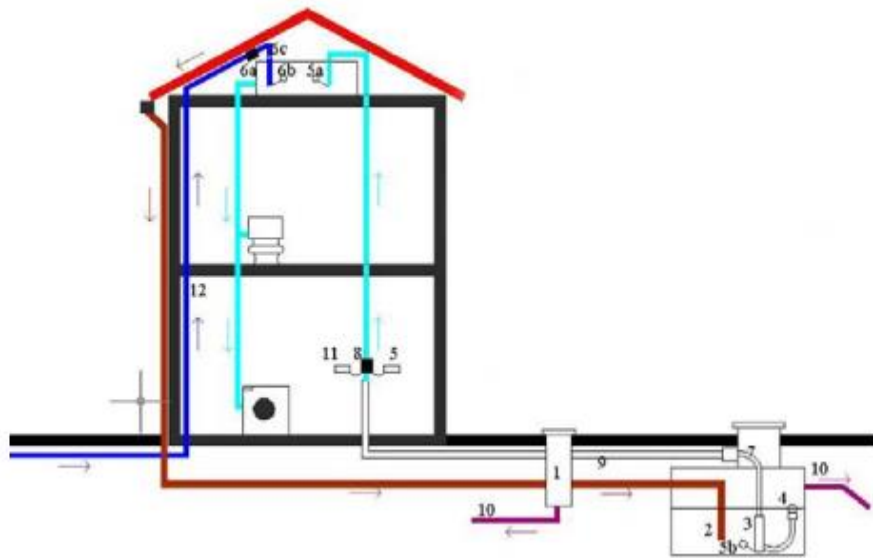
Figure 30. Distribution by gravity (Şahin and Manioglu, 2011)
