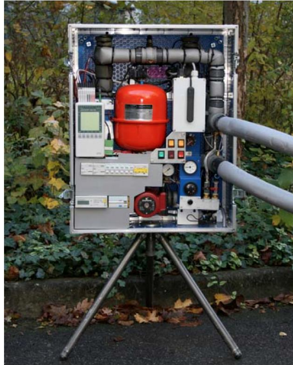
Figure A.11 : Thermal response test unit of EPFL, Switzerland. Photo: EPFL.
