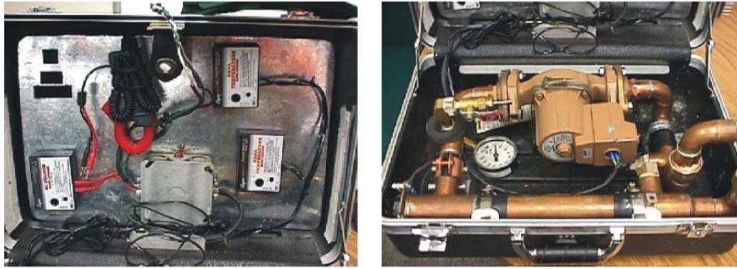
Figure A.9 : Suitcase thermal response test unit of TriSun Construction, Oklahoma. Photo: Jeffrey Spitler.
