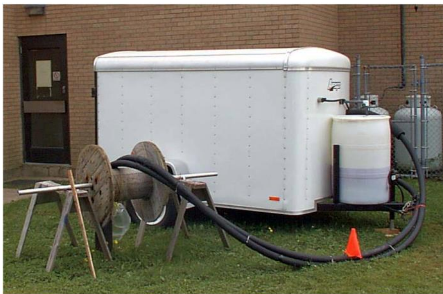
Figure A.2 : Canadian thermal response test rig. Photo: Environment Canada.
