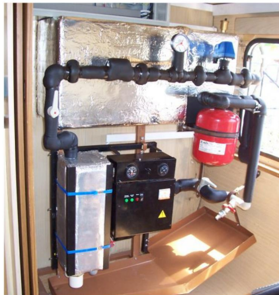
Figure A.12 : Thermal response test unit used in Bulgaria (Georgiev et al., 2009).
