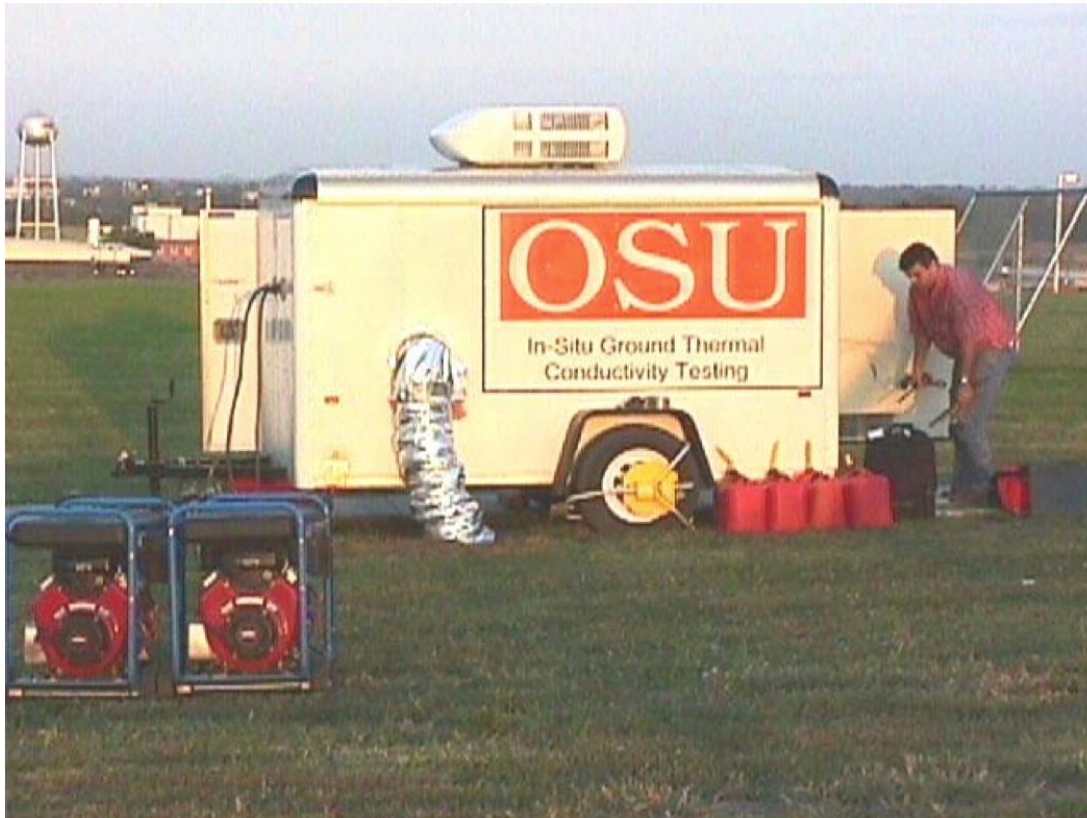
Figure A.7 : Oklahoma State University thermal response test rig. Photo: Jeffrey Spitler.
