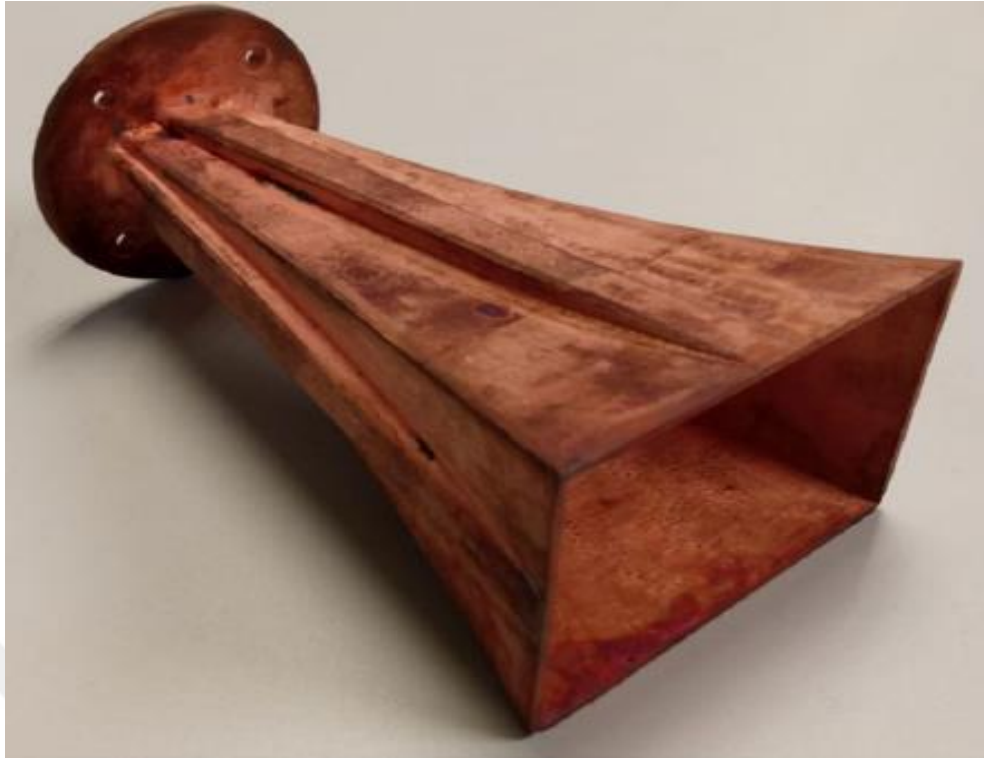
Figure 2.4. 3D-printed antenna prototype (Bachiller et al., 2023)
