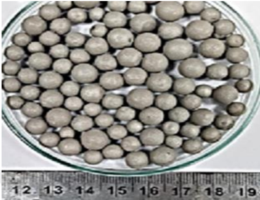
Figure 2.14. The aluminium-coated expanded polystyrene spherical structures (Srivastava et al., 2023)
