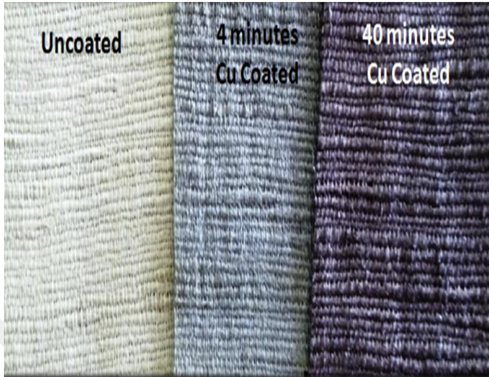
Figure 2.13. The appearance of the polyester-silk blend before and after coating (Rani et al., 2017)
