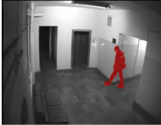
Figure 2.2. Simple background modeling motion detection [20].
