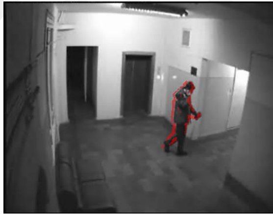
Figure 2.1. Two frames difference motion detection [20].
