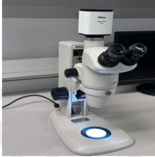
Şekil 3.14: Nikon SMZ745T (Nikon Instruments Europe BV, Hollanda).
