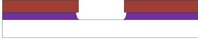
Figure 3.9: Undercuts formed during wet etch of \text{SiO}_2 .
