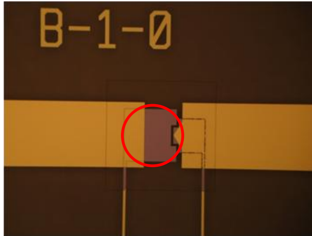
Figure 4.18: Position of the droplet after the actuation is shown by the red circle.
