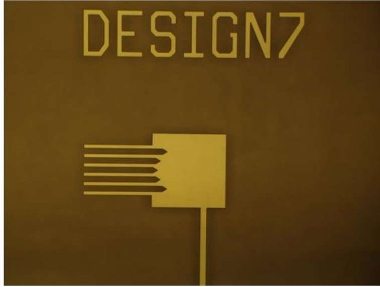
Figure 3.5: Sample device with coated and patterned Cr electrode. The contact pad below is not shown.
