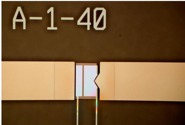
Figure 4.26: Successful patterning of the Teflon AF layer using Zonyl FSN as the surfactant with optimized photolithography parameters.
