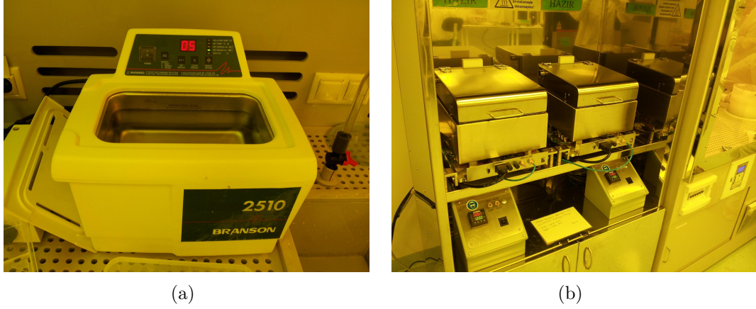
Figure 3.2: (a) Samples were first ultrasonically degreased in a 5-min acetone ( (\text{CH}_3)_2\text{CO} ) bath, followed by a 5-min isopropyl alcohol ( (\text{CH}_3)_2\text{CHOH} ) bath. (b) They were dehydration-baked on a controlled hot-plate at 120^\circ\text{C} for 5 min.
