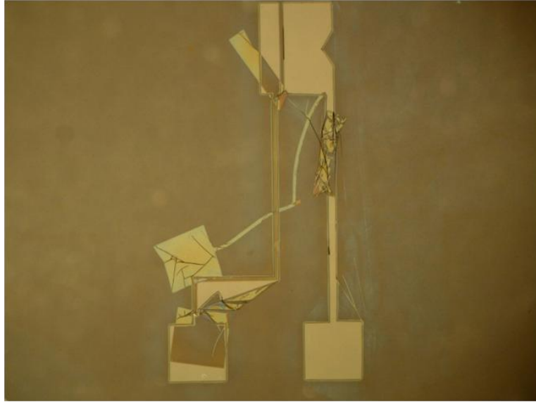
Figure 4.21: Unsuccessful Teflon patterning (Lift Off). Photoresist used was AZ 5214 with a thickness of 1.4\ \mu\text{m} .
