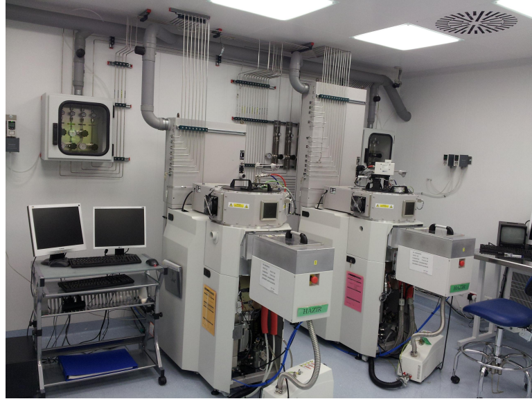
Figure 3.10: ICP system utilized for dry etching processes.
