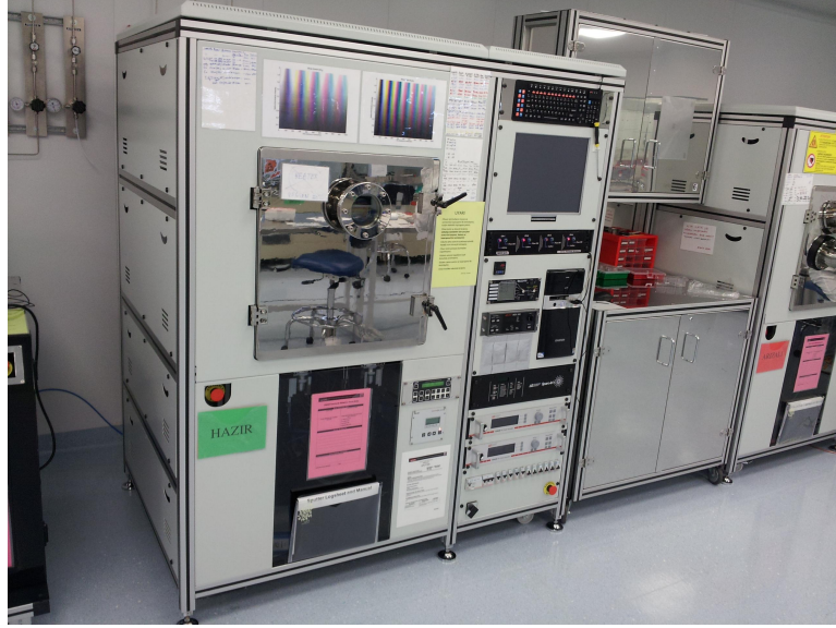
Figure 3.3: VAKSIS Sputter system used for metallic coating processes in this work.
