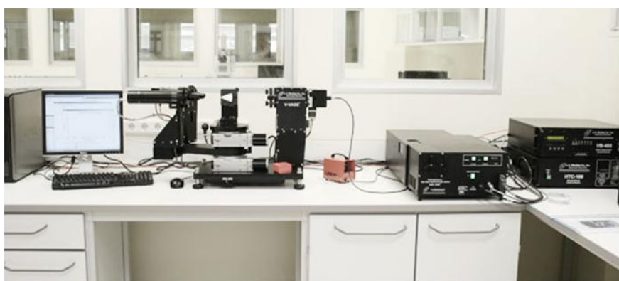
Figure 3.7: J. A. Woolam V-VASE spectroscopic ellipsometer.
