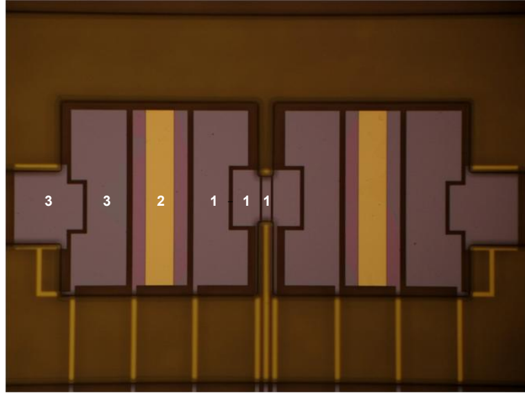
Figure 4.11: Optical microscope image of the fabricated device designed for droplet merging and separation experiments.
