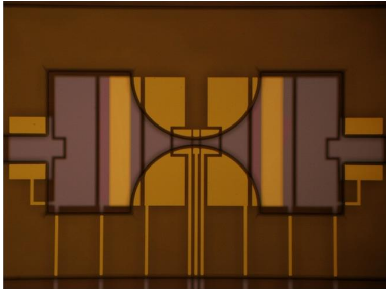
Figure 4.15: Optical microscope image of the fabricated LS-MEMS device having a graded neck region.
