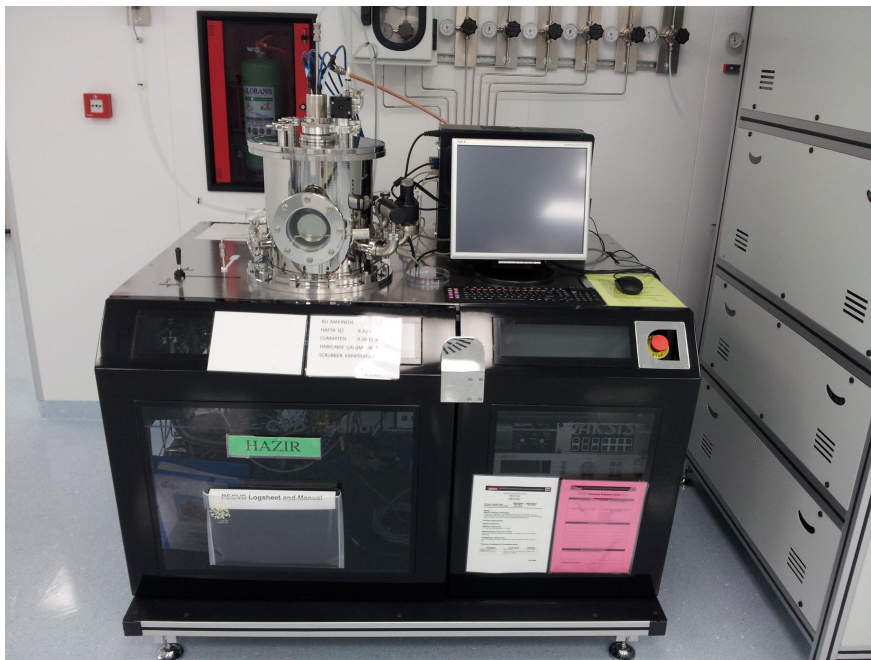
Figure 3.6: VAKSIS PECVD system used for dielectric coating processes in this work.
