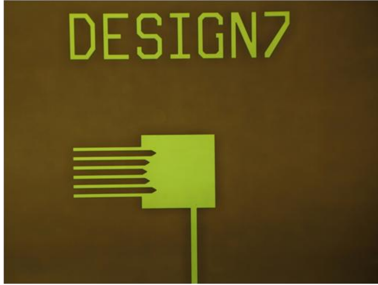
Figure 3.11: Sample device with coated and patterned \text{SiO}_2 dielectric layer.
