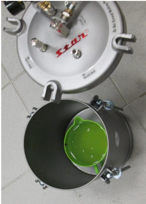
Figure 3.9 (m-o) Disassembled components of the through-thickness permeability measurement setup.
