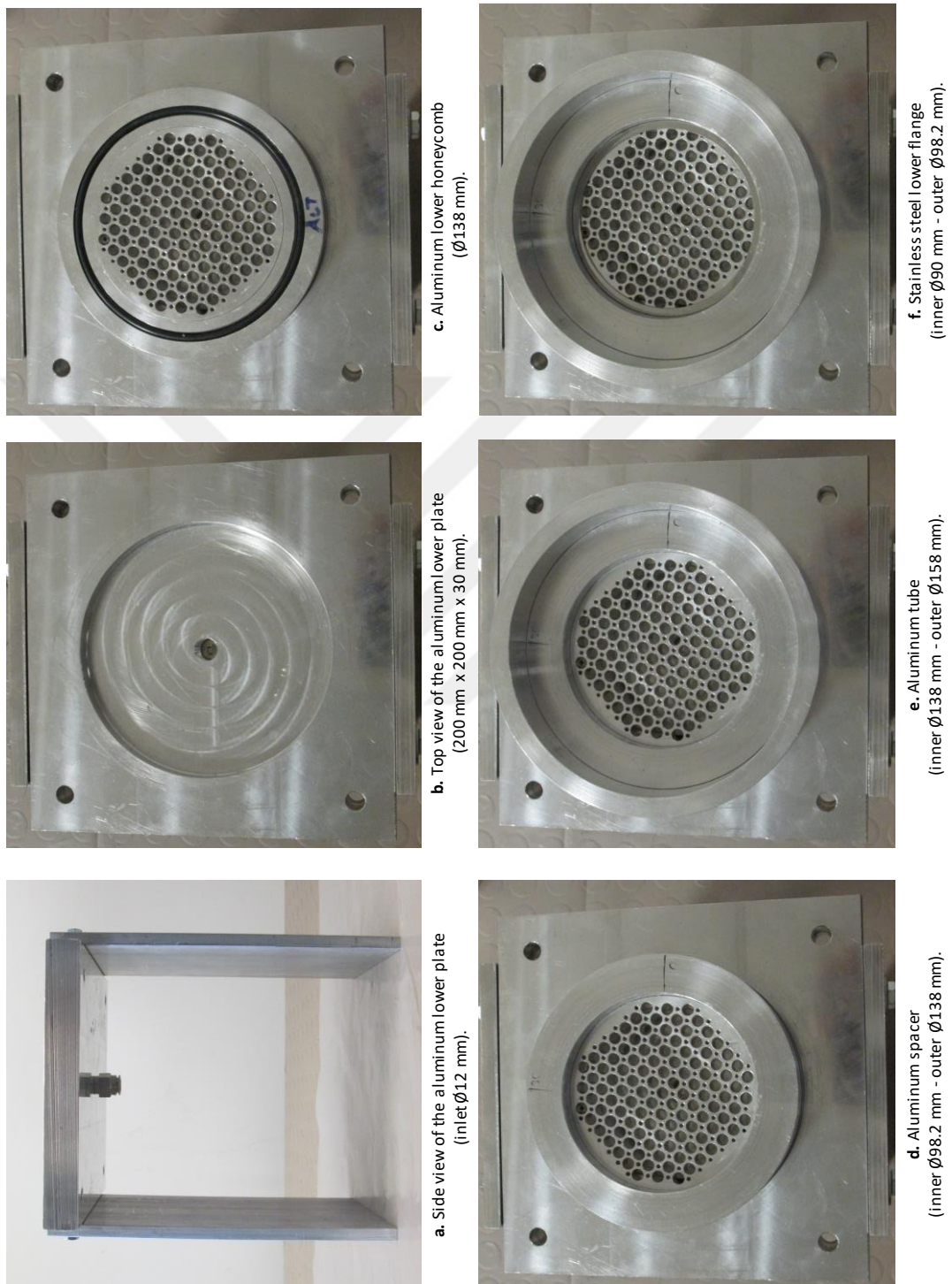
Figure 3.9 (a-f) Disassembled components of the through-thickness permeability measurement setup.
