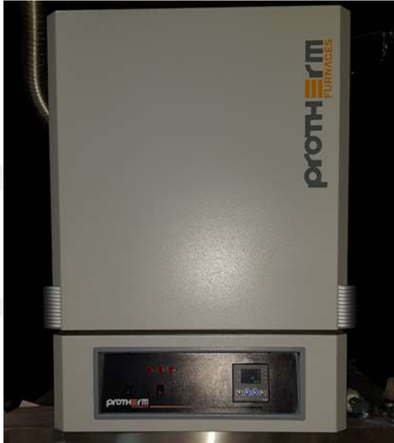
Figure 3.4. Protherm brand ash furnace.
