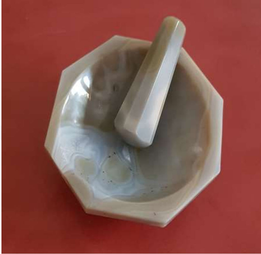
Figure 3.2. Agate mortar which was used to pestle all chemical inputs and output materials
