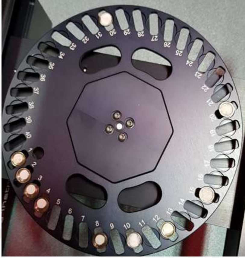
Figure 3.7. Sample cups(planchets) on the sample wheel(carousel).
