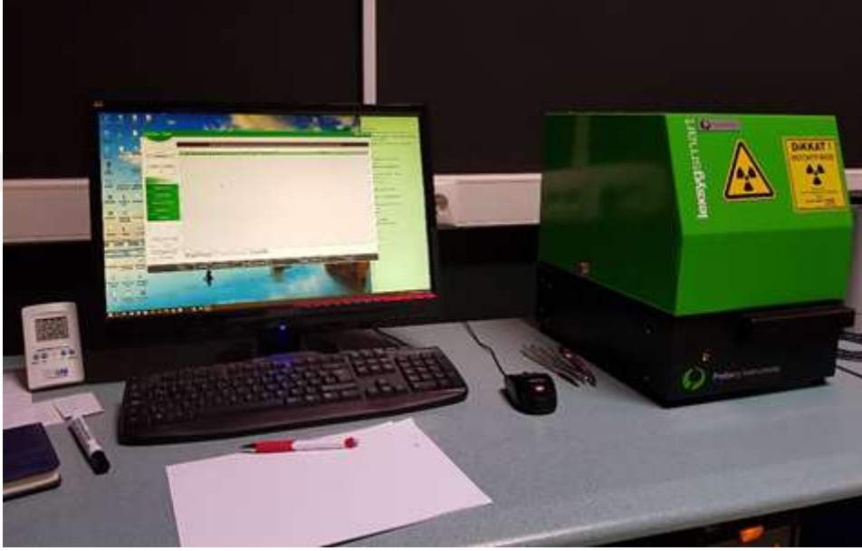
Figure 3.6. Freiberg Instruments Lexyg Smart TL/OSL reader system.
