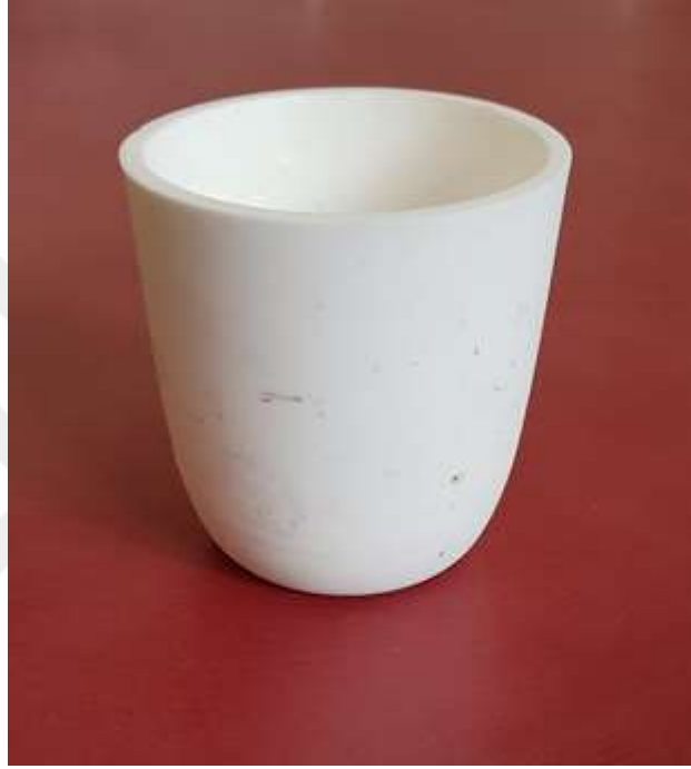
Figure 3.3. One of the alumina crucibles which were used for the syntheses.
