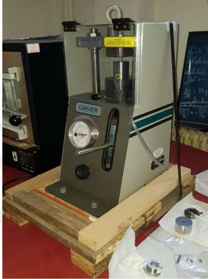
Figure 3.5. Carver brand hydraulic press and its parts.
