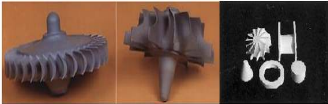
Figure 1.10 Ceramic products formed by gel casting [52]
