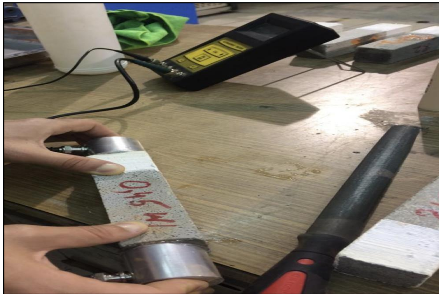
Figure 3.10. Ultrasonic pulse velocity (UPV) test setup.
