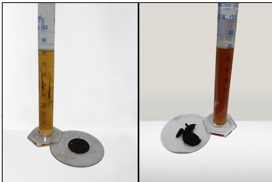
Figure 4.2. Liquid and solid outputs of HTC at 180°C (left) and 250°C (right).
