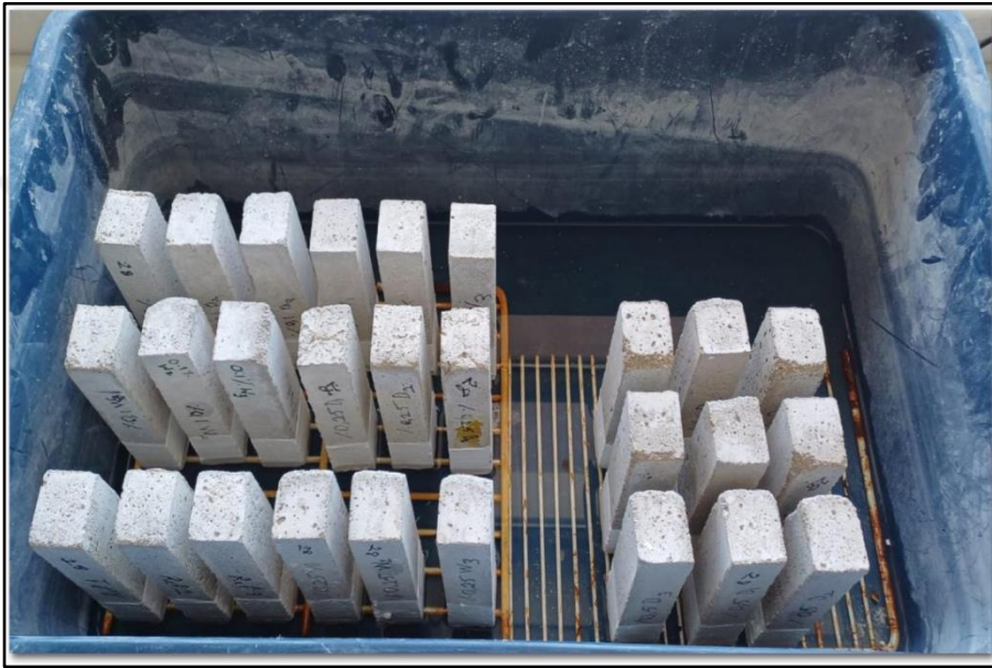
Figure 3.9. Experimental setup for capillary water absorption testing.
