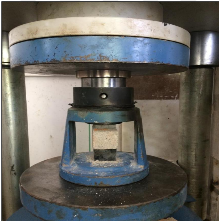
Figure 3.11. Compressive strength test setup for evaluating the load-bearing capacity of samples.
