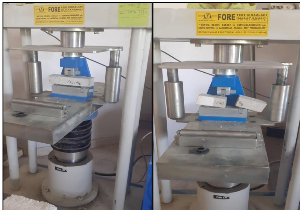
Figure 3.12. Flexural strength test setup: before (intact) and after fracture (broken).
