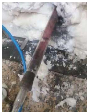
Figure 6.5. Reduction with hydrogen in quartz glass tube reactor
