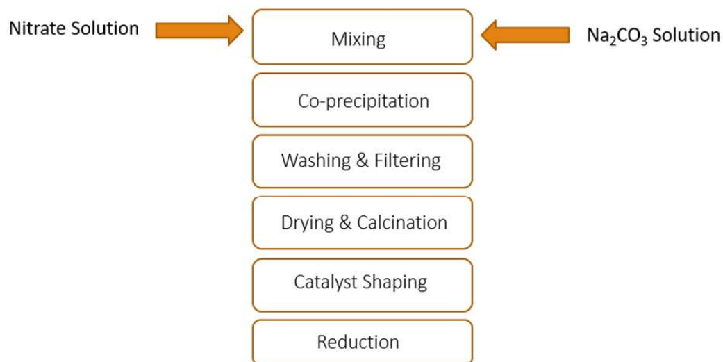
Figure 4.1. Co-precipitation method procedure
