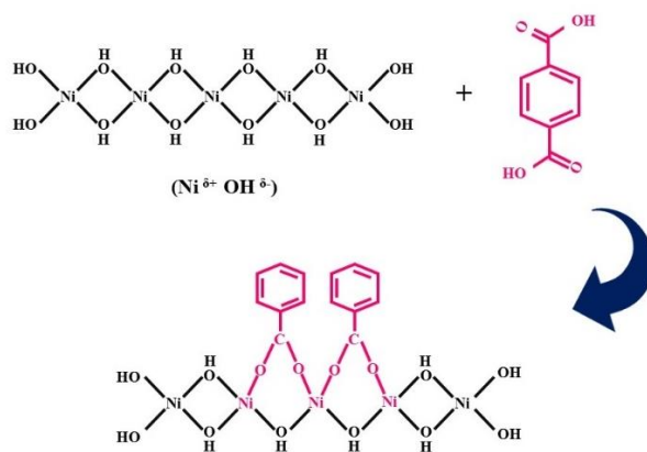
Figure C1. The coupling mechanism of \text{Ni}(\text{OH})_2 as the dominant phase of NCF with Ni-BDC ligand.
