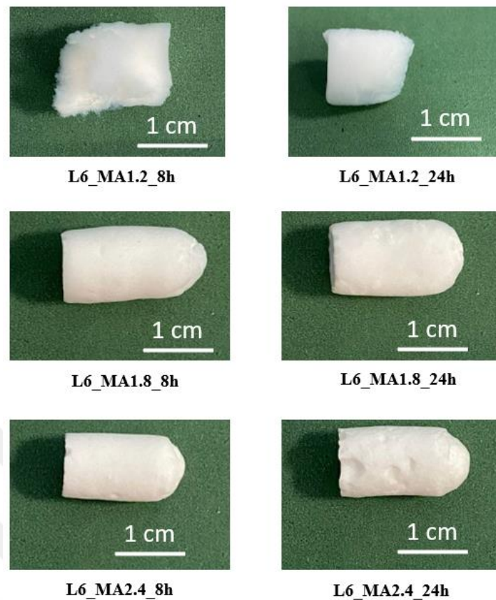
Figure 4.5. Photos of CMC aerogels from 6 wt % CMC solutions.
