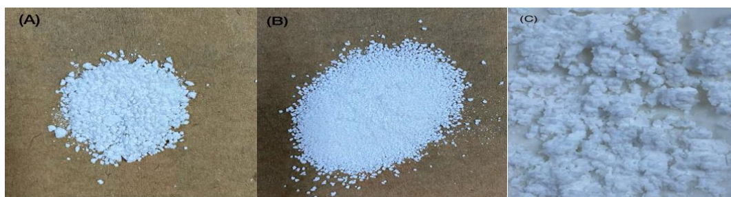
Figure 9: Poly(HEMA- co -EGDMA)(S3), A: (F1) >710 \mu\text{m} . B: (F2) 710-212 \mu\text{m} . C: (S3)Before Separation by Sieves.
