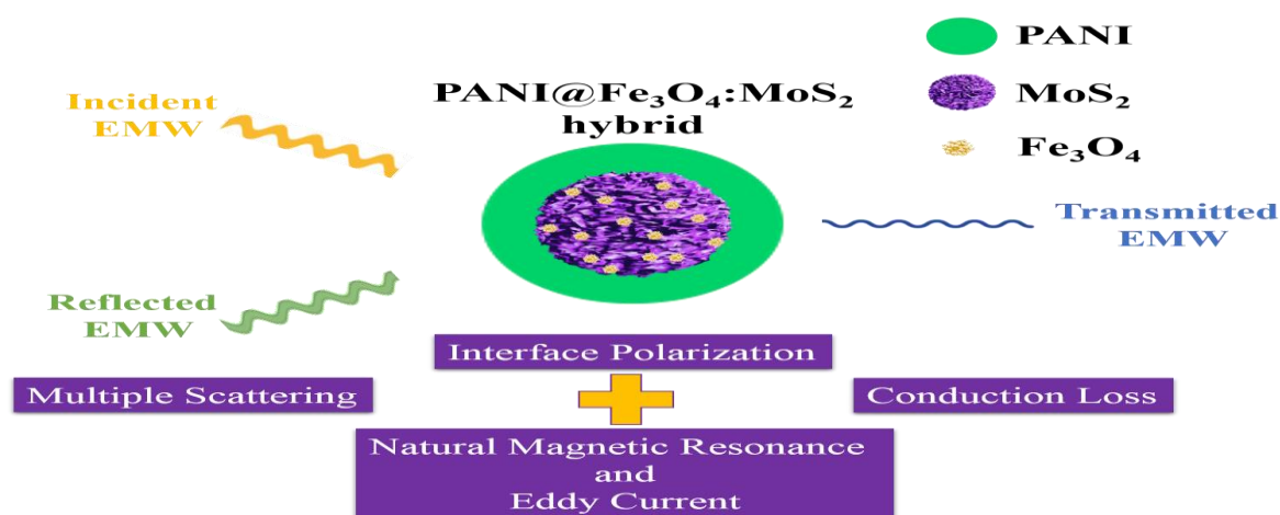
Figure 4.18. Schematic representation of the reflection loss mechanism of PANI@Fe 3 O 4 :MoS 2 hybrid structure.
