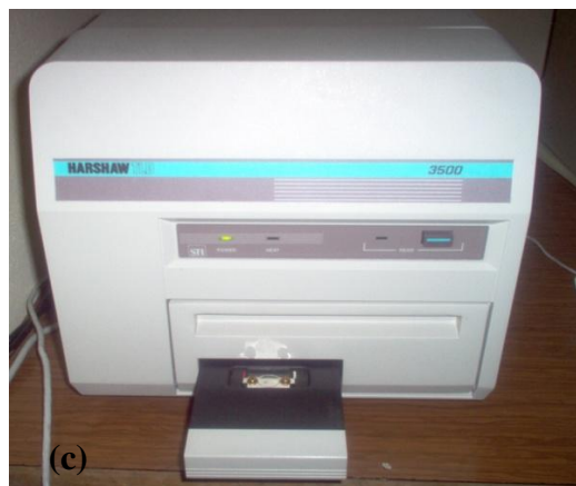
Figure 4.3 Experimental equipments (a) ^{90}\text{Sr} - ^{90}\text{Y} \beta -source (b) 9010 Optical Dating System (c) Harshaw TLD System 3500.
