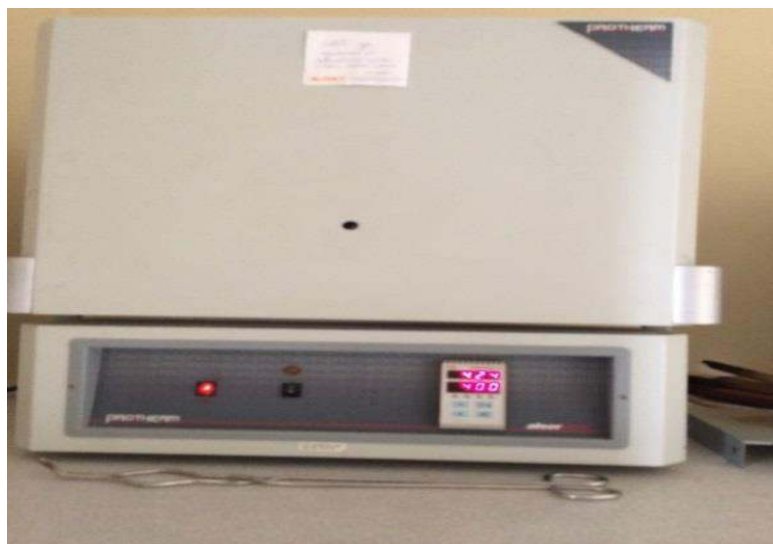
Figure 4.5 Nuve FN 501 type electrical oven
