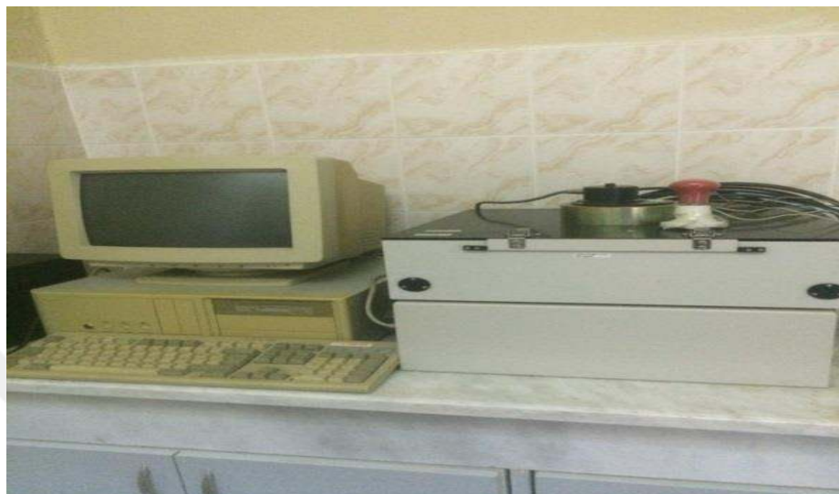
Figure 4.1 Radiation source of beta rays a ^{90}\text{Sr} - ^{90}\text{Y} source ( \approx 0.04 Gy/s).
