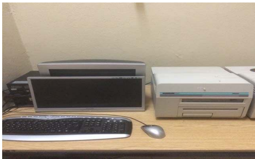
Figure 4.2 QS 3500 Harshaw TLD reader
