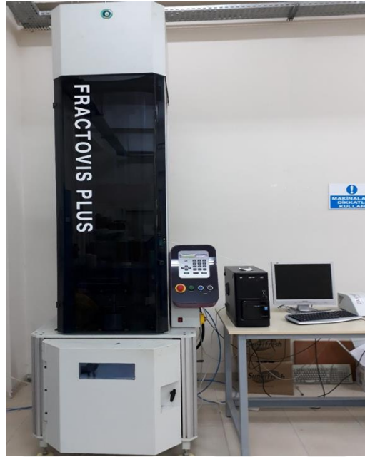
Figure 2.5 Ceast Fractovis-Plus impact test machine (Personal archive, 2019)
