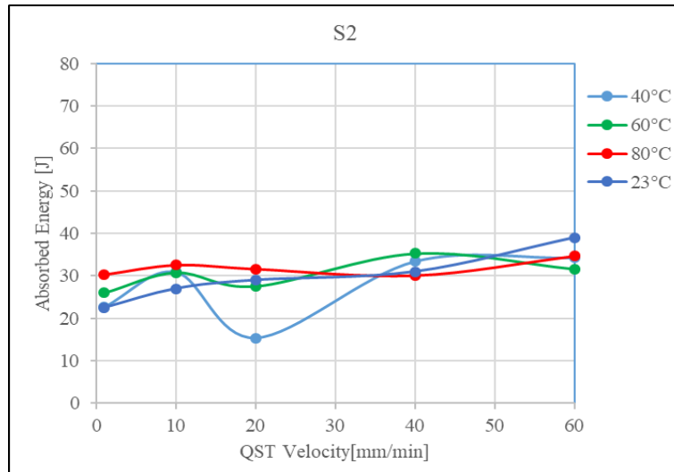
Figure 3.59 Absorbed energy versus QST velocity diagram under quasi-static test with flat nose penetrator S2 glass/epoxy composite
