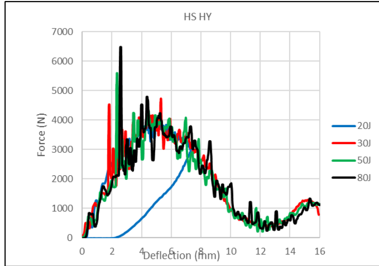
Figure 3.13 Force-deflection diagrams for hybrid carbon-kevlar/epoxy hemispherical nose in impact test at 23 °C
