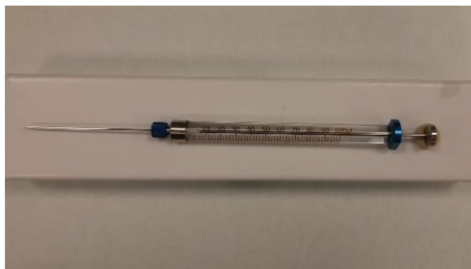
Figure 3.5: Gas Tight Syringe
