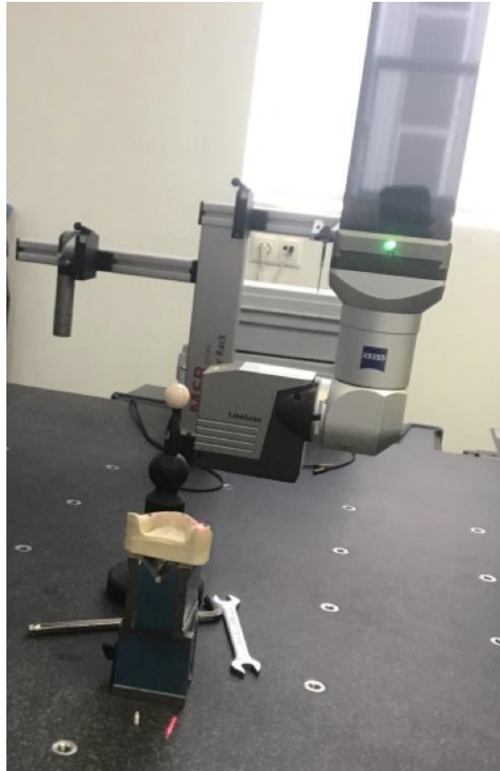
Figure3. 5 Scanning the study model with a reference scanner
