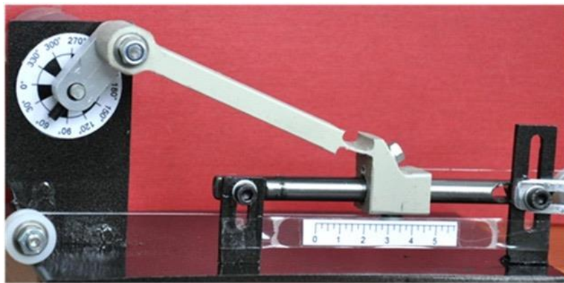
Figure 1.3. Manufactured partially compliant slider-crank mechanism [16]
