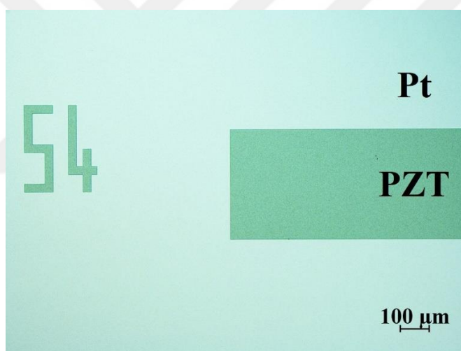
Figure 3.2. Microscopic image after PLD-PZT etch.
