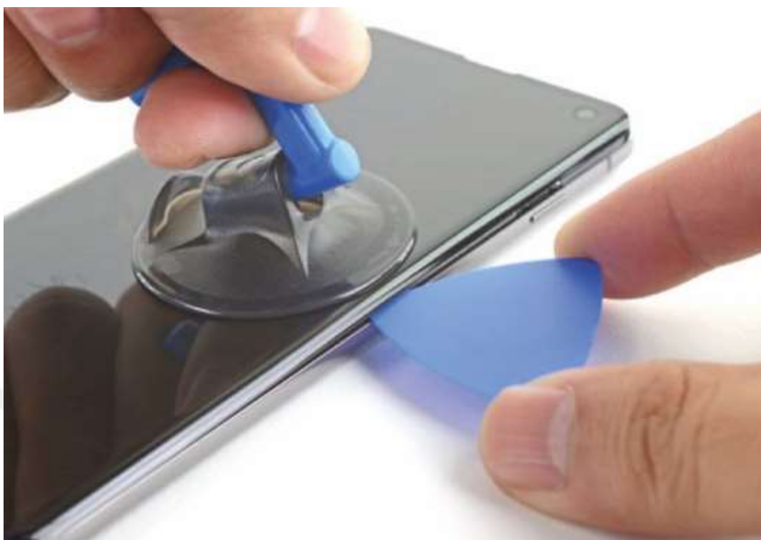
Figure 4.34 Representative image for phone screen removal with proper equipment (iFixit.com, n.d.).
