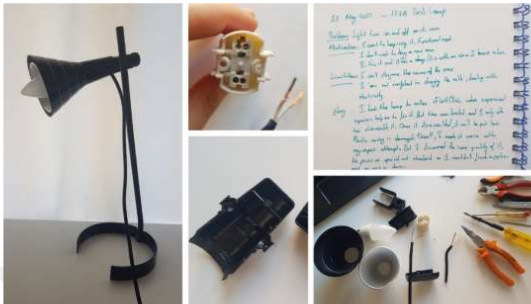
Figure 3.2 Collage from my product care photo album and notes about the repair process of my desk lamp.
