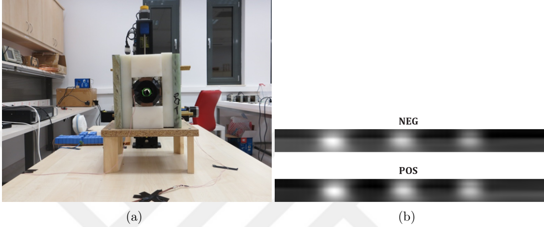
Figure 4.6: (a) The MPI Scanner developed in our lab. (b) The standard x-space reconstructed MPI images from negative and positive half-cycles.
