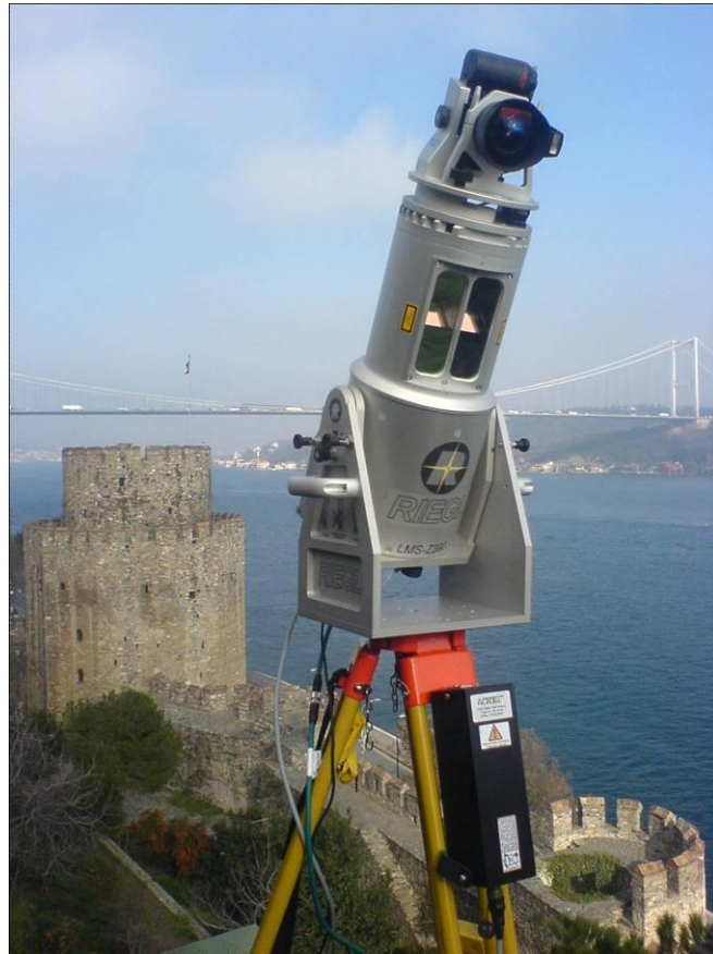
Şekil 4.33 Lazer tarayıcı (Terrestrial laser scanning, (b.t). 2012, www.riegl.com).
