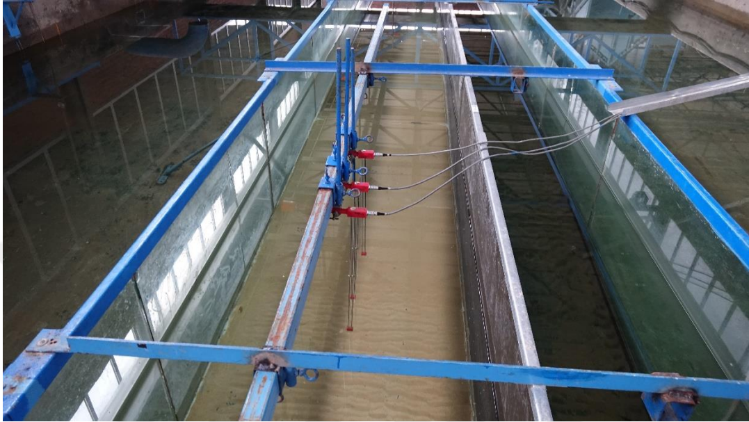
Figure 3.7. The group of wave gauges placed at the slope
