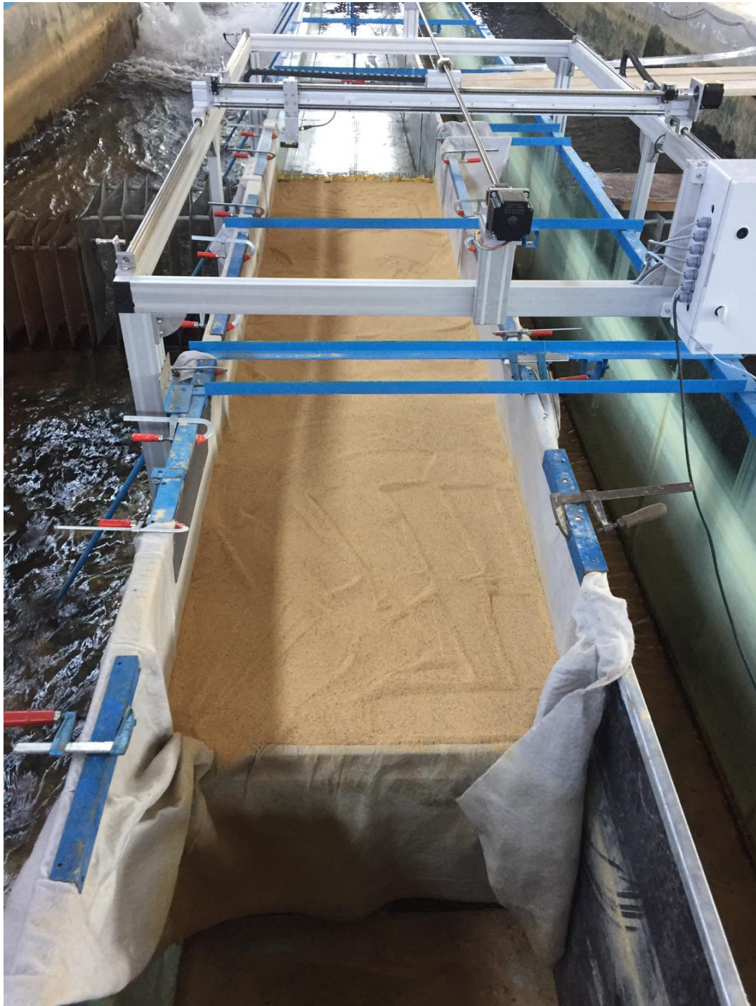
Figure 3.9. Experimental setup with the computer-controlled bottom profiler
