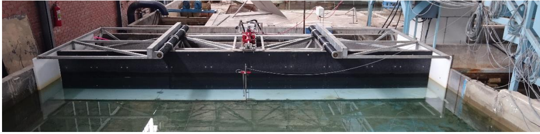
Figure 3.2. Piston type wave generator
