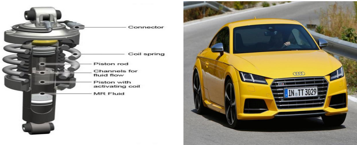
Figure 2-15: First MagneRide™ introduced in 2002 (Left), the third-gen Audi TT launched with MagneRide™ Dampers(Right) [23].
