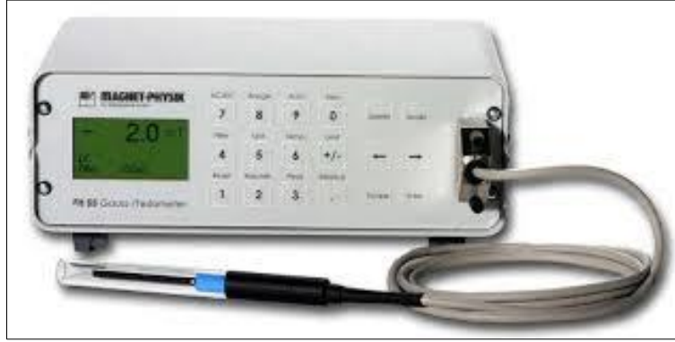
Figure 3-3: Gauss/Teslameter used for magnetic flux density measurement.
