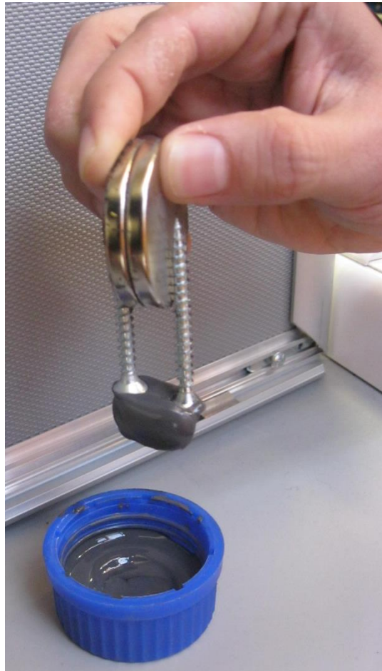
Figure 2-1: MR fluid in liquid form in the absence of magnetic field turns solid when magnetic field is applied .
