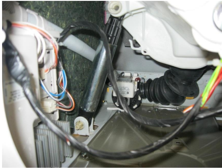
Figure 2-28: Rear view of front loaded washing machine. Passive damper is visible with one end attached to the base and other end connected to suspended tub.
