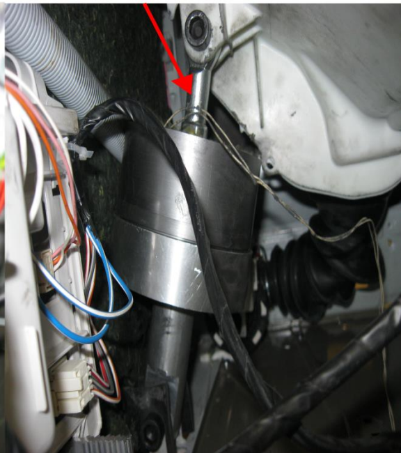
Figure 7-4: Passive and MR dampers are installed separately in washing machine.
