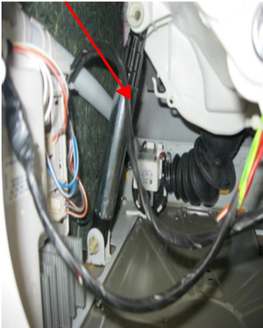
Figure 7-4: Passive and MR dampers are installed separately in washing machine.
