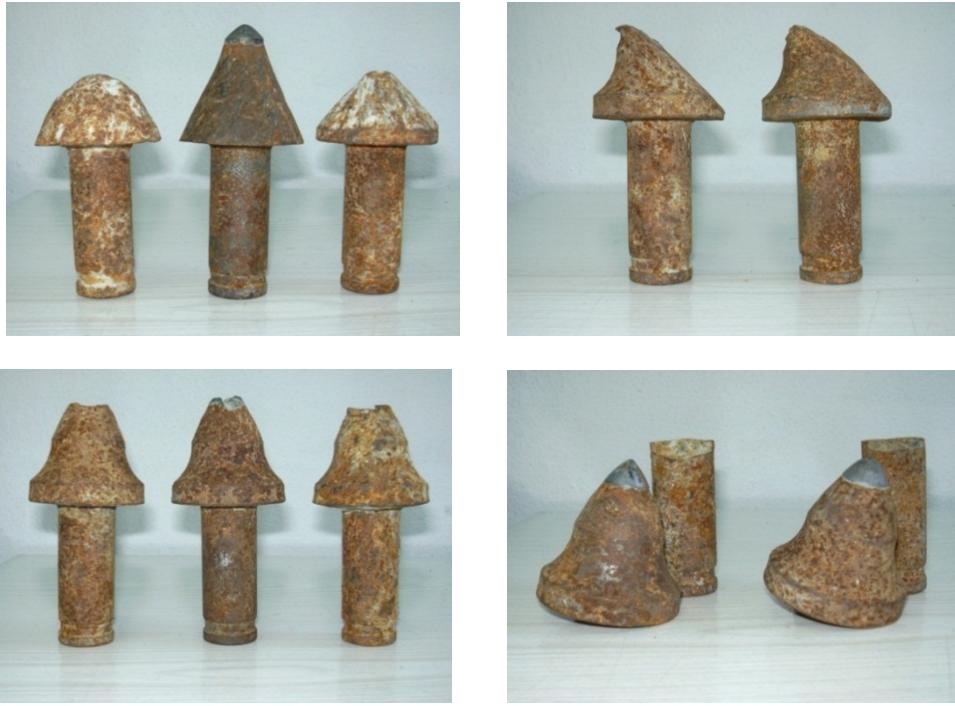
Figure 2.16 : Cutter wear classification in Kucuksu Tunnel.
