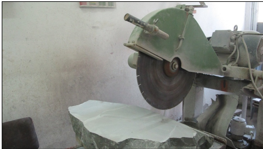
Figure 3.1 : Saw used in preparation of rock samples.
