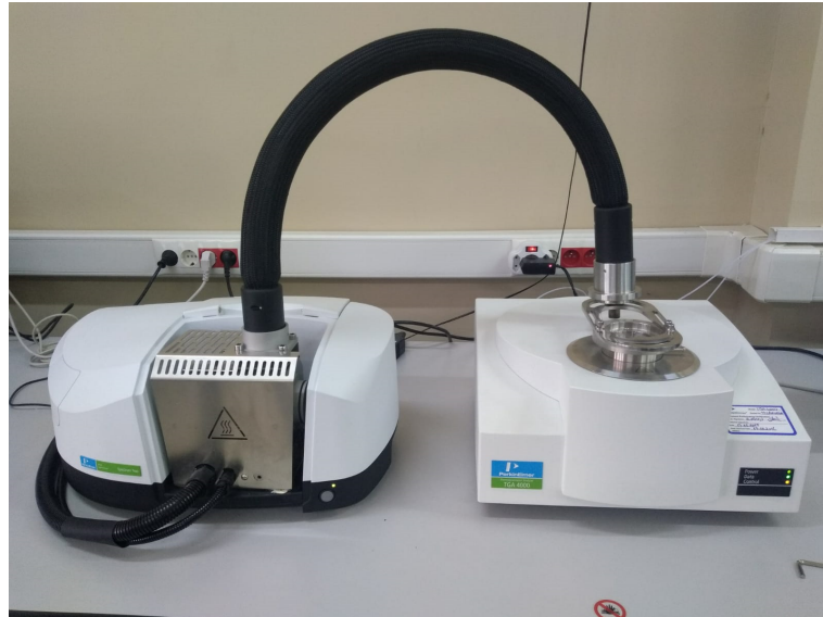
Figure 3.7: Perkin Elmer Pyris STA 4000 Thermogravimetric analyzer (right) equipped with Fourier-transform infrared spectrometer (left) at RÜZGEM.
